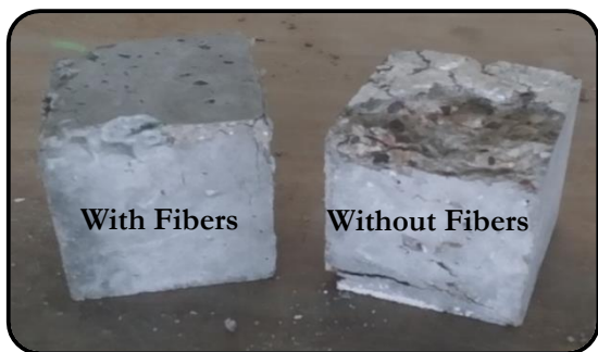
Figure (8): Shape of failure under compression load
