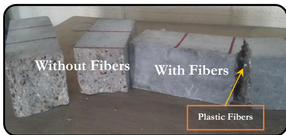
Figure (10): Shape of failure under bending
