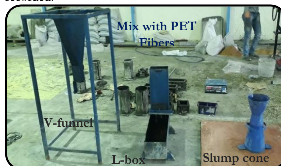
Figure (2): Preparation of instruments for SCC tests
