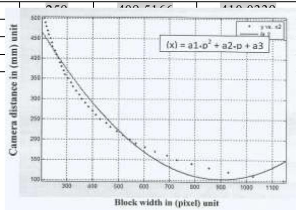
**Figure (6) the relation of camera distances and widths of block and their fitting curve**
