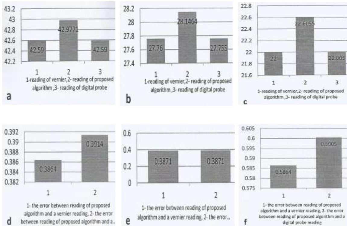
Figure(15) (a,b,c) comparison of digital vernier, scanning program and digital probe reading, (d,e,f) comparison the error of dimension for triangular shape
