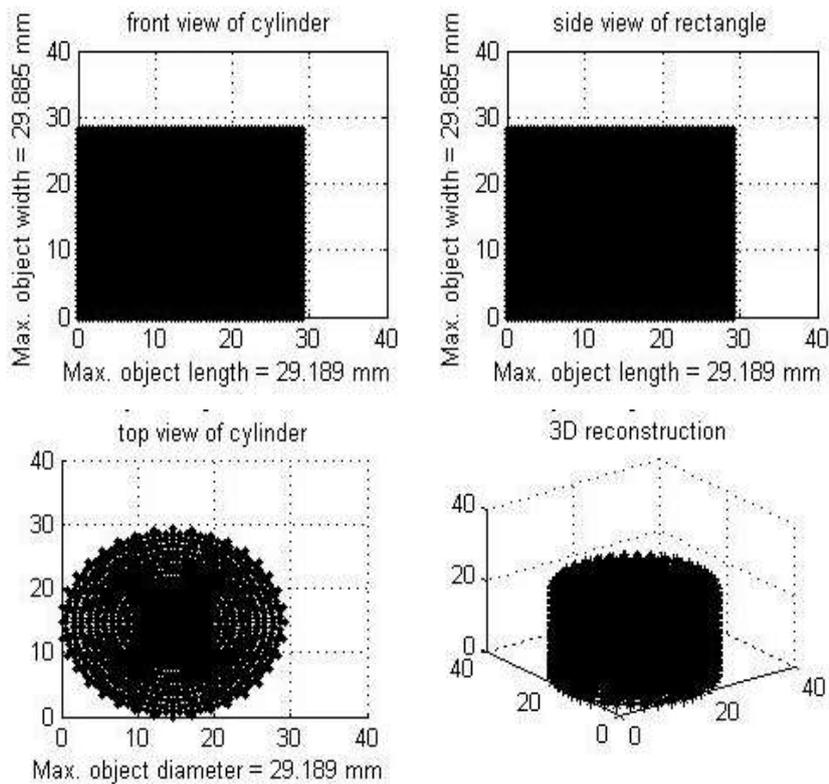
Figure (17) 3D Reconstruction of cylindrical shape with its dimensions and its projections.
