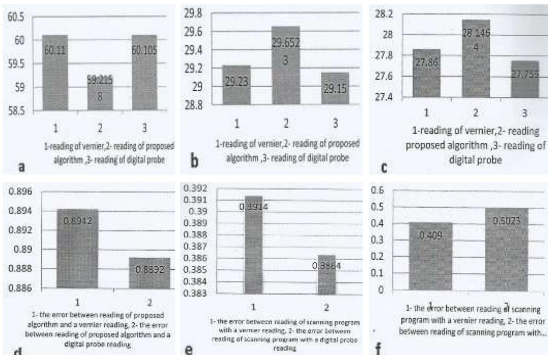
Figure (13) (a,b,c) comparison of digital vernier, scanning program and digital probe reading, (d,e,f) comparison the error of dimension for rectangular shape
