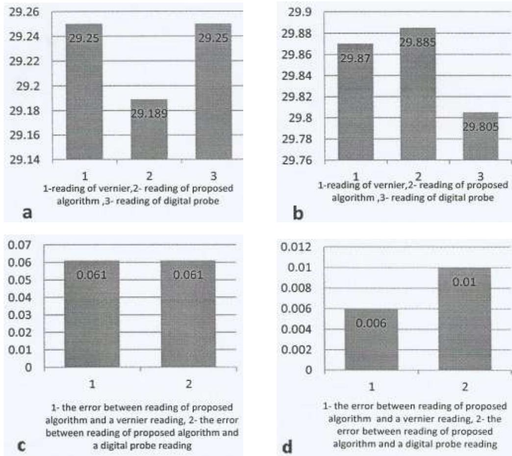
Figure(18) (a,c) comparison of digital vernier, scanning program and digital probe reading, (b,d) comparison the error of dimension for cylindrical shape
