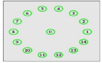
Figure 1 Star network topology (node 0 is a coordinator, nodes (1-14) are end devices)
