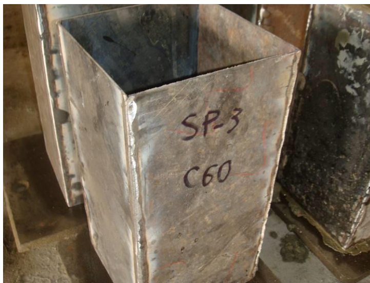
Figure (6): Specimen layout and weld detailing.
