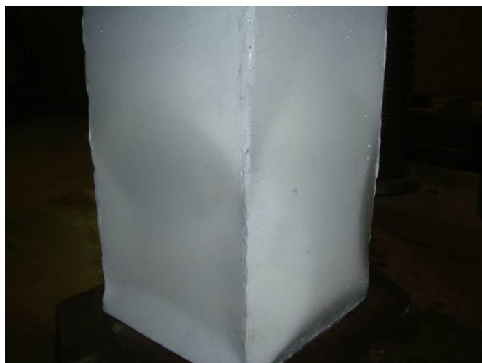
a) Experimental Buckling Mode.
