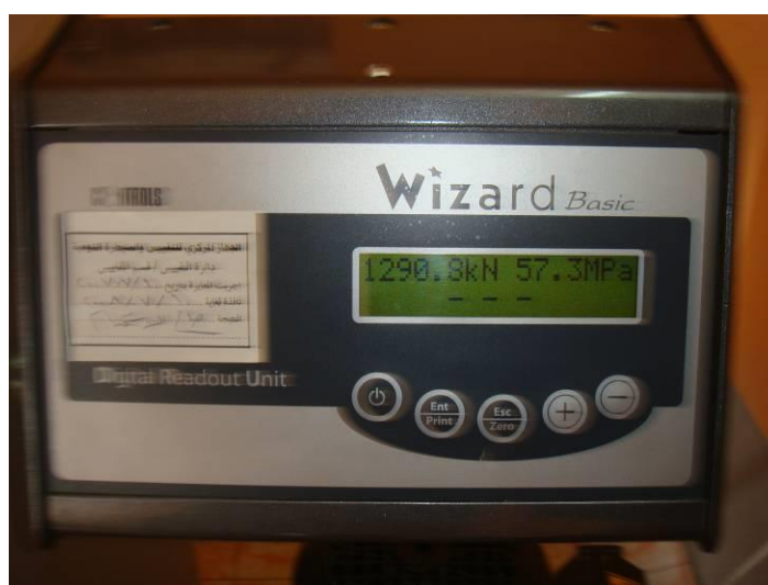
Figure (9): Apparatus Recording the Ultimate Load Capacity of Specimen SP3.
