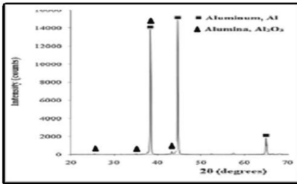
Figure 2. XRD pattern of samples
