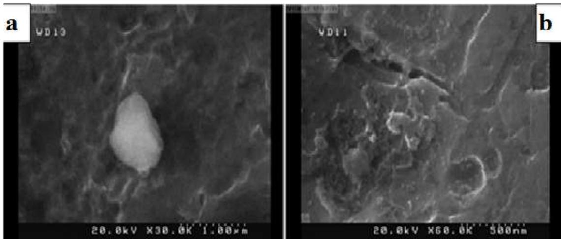
Figure 4 SEM images illustrated effects of stirring velocity on alumina particle size
