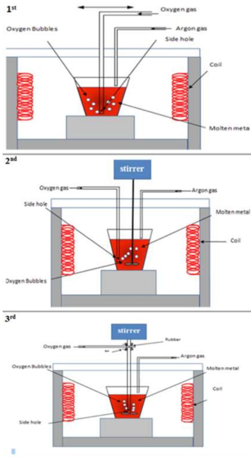
Figure. 1 illustrated 1<sup>st</sup>, 2<sup>nd</sup> and 3<sup>rd</sup> stirring methods
