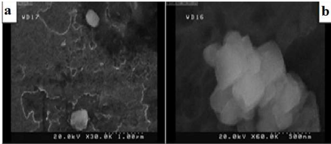
**Figure 5 SEM images Illustrated alumina particle size a) at 1770 rpm stirring velocity, b) at 2280 rpm stirring velocity with hole dia.600μm by third stirring method**
