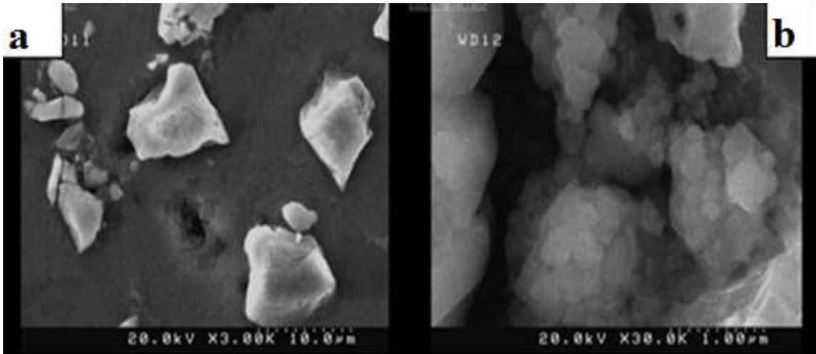
Figure 3 SEM images Illustrated effects of side hole dia. On alumina particles size
