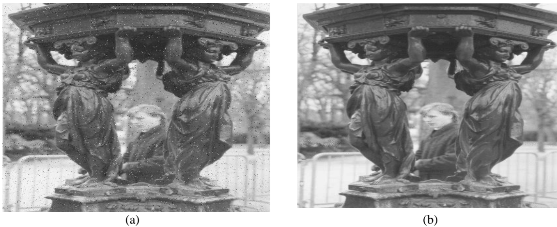
figure 2 : picture(a) an image with noise and (b) the image after Gaussian filter smoothing
