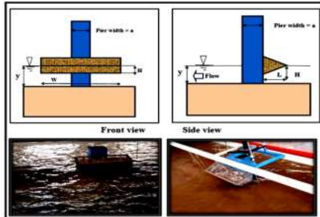
Figure (6): Layout of the wedge debris, Run3.
