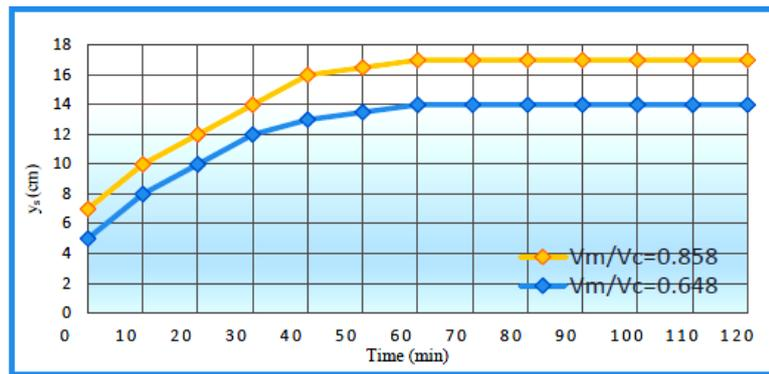
Figure (13): Development of scour depth with the time.
