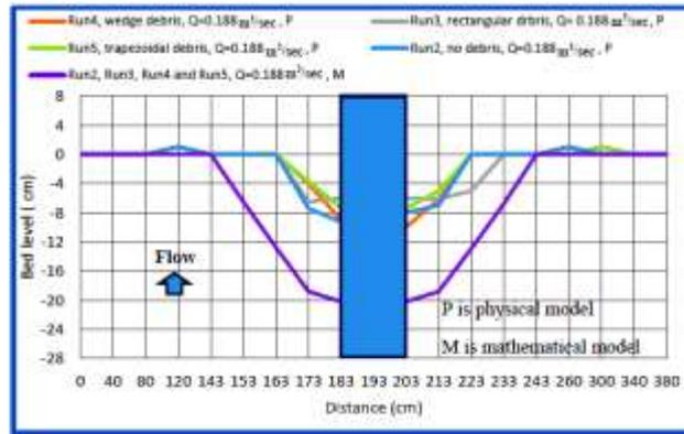
Figure (19): Effect of different shapes of floating debris on the scour depth (front view).
