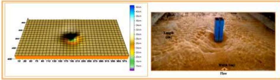
Figure (18): Scour hole for Run5, trapezoidal debris and  $Q=0.188 \text{ m}^3/\text{sec}$ .
