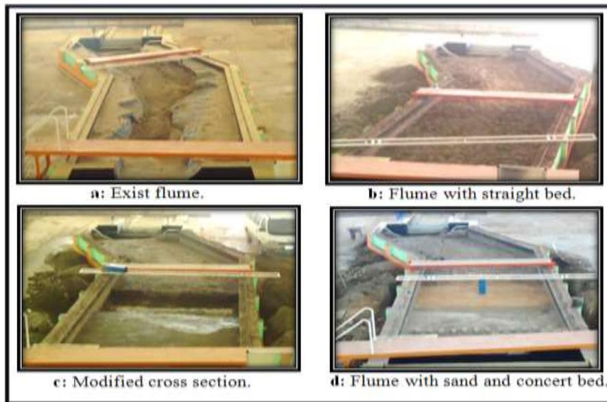
Figure (2): Stages of modifying the laboratory flume.
