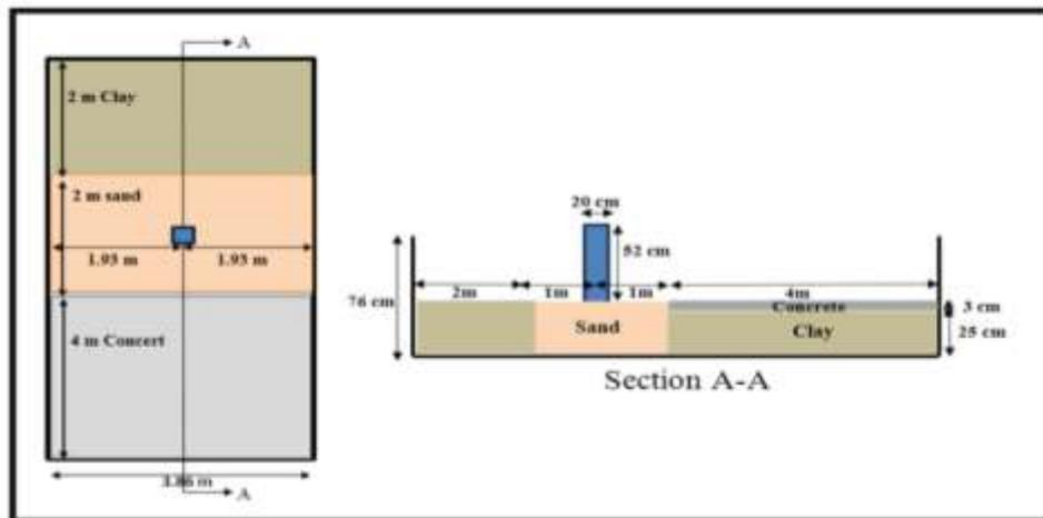
**Figure (3): Layout of fabricated steel pier within the flume.**
