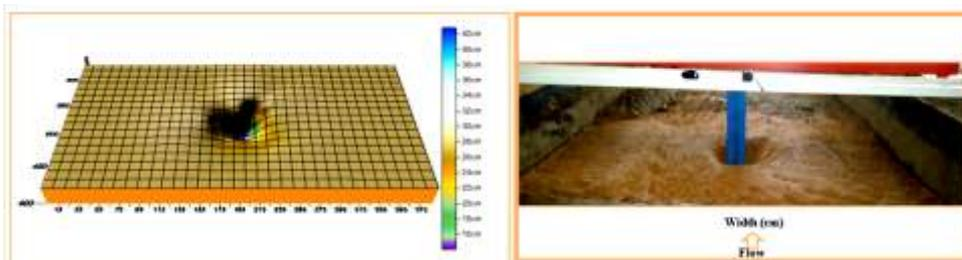
Figure (14): scour hole for Run1, no debris and  $Q=0.249\text{m}^3/\text{sec}$ .
