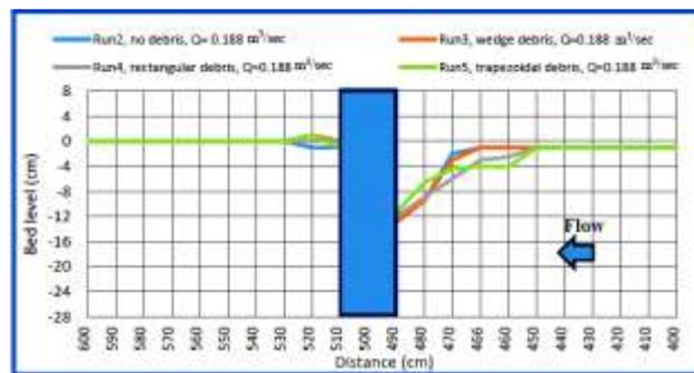
Figure (20): Effect of different shapes of floating debris on the scour depth (side view).
