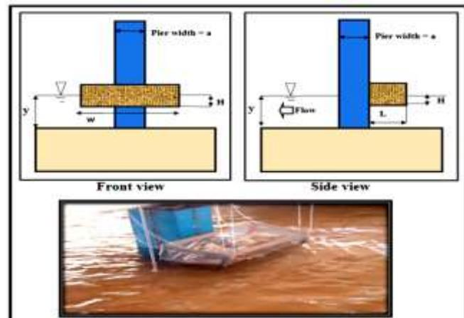
Figure (7): Layout of the rectangular debris, Run4.
