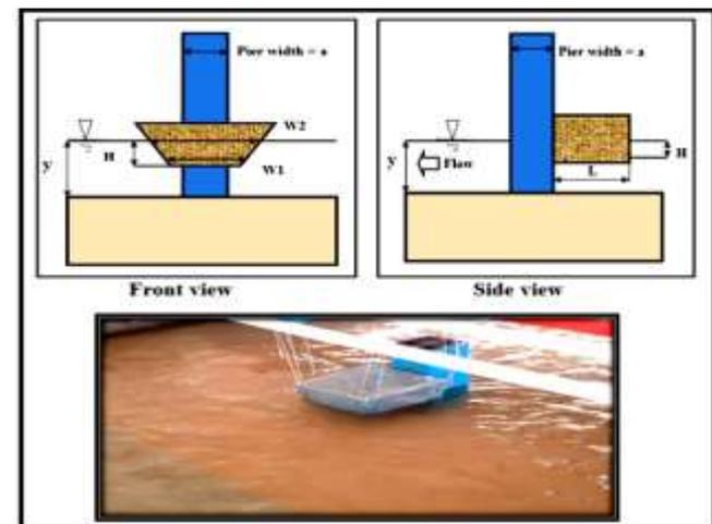
Figure (8): Layout of the trapezoidal debris, Run5.
