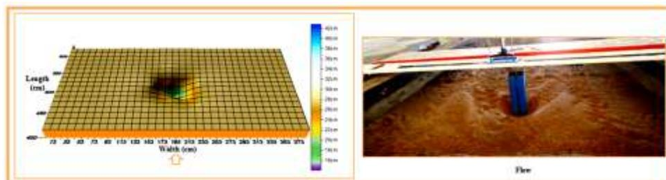
Figure (15): scour hole for Run2, no debris and  $Q=0.188\text{m}^3/\text{sec}$ .
