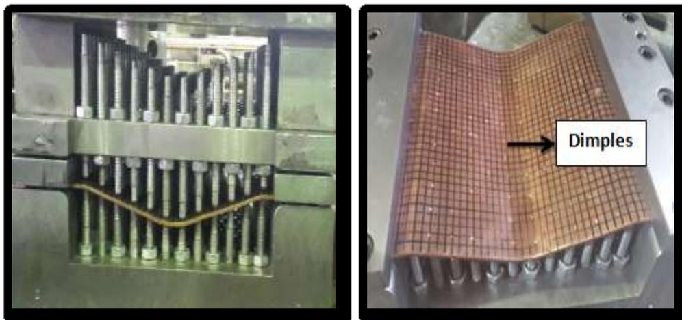
**Figure (11): Final product formed by MPF process without rubber.**
