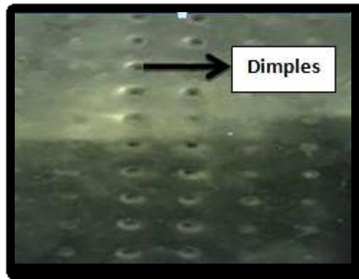
Figure (12): Rubber deformation after MPF process
