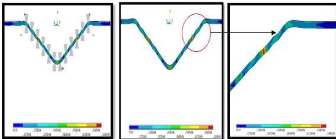
**Figure (15): Final product formed by MPF without rubber**
