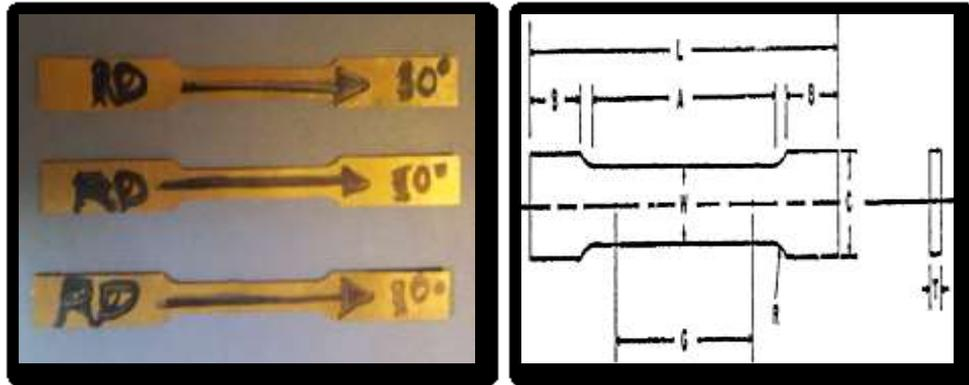
Figure (8): Rectangular cross section tensile test specimen, ASTM E8-M.[7]
