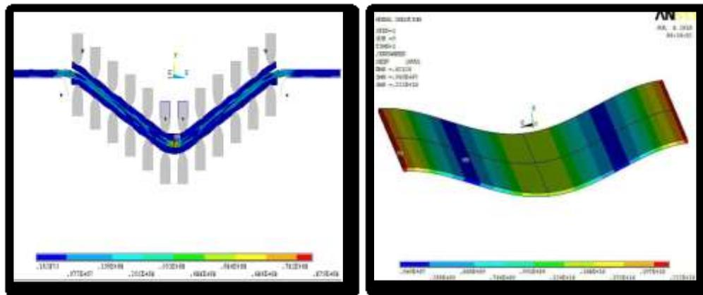
**Figure (14): MPF with rubber (a) 2-D modeling, (b) 3-D modeling**
