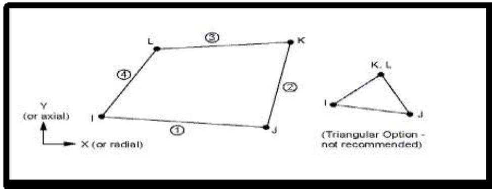
Figure (4): Element 182 geometry
