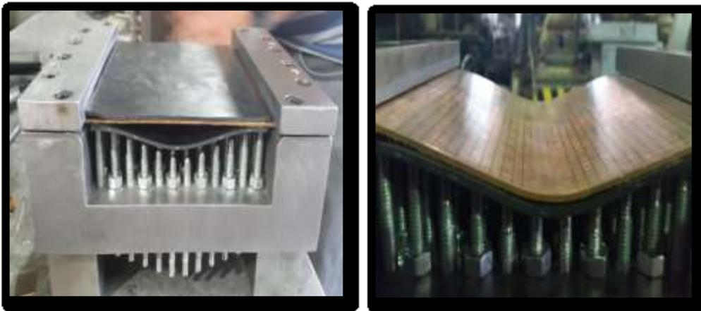
**Figure (10): Final product formed by MPF process with rubber.**
