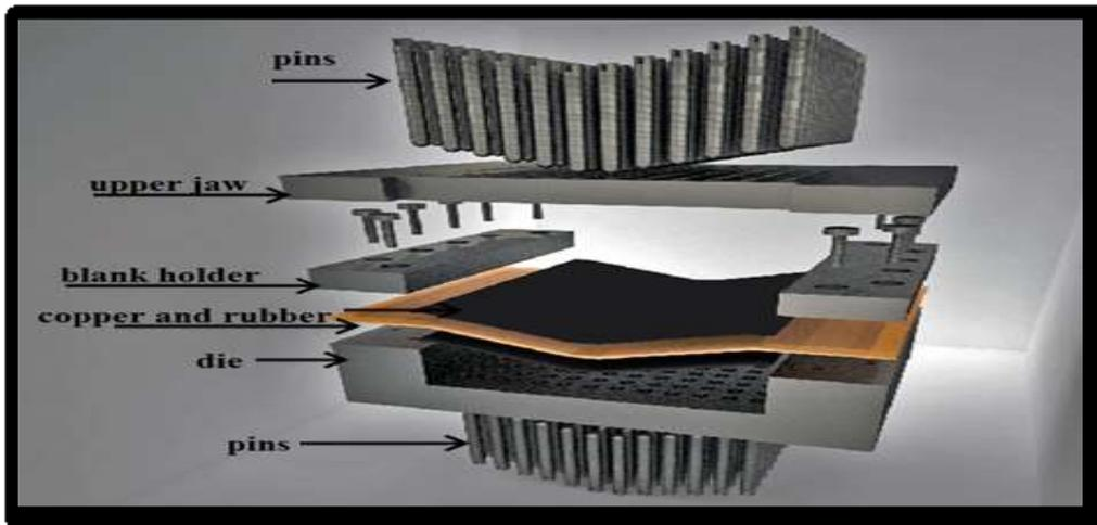
Figure (6): MPF die and pins design
