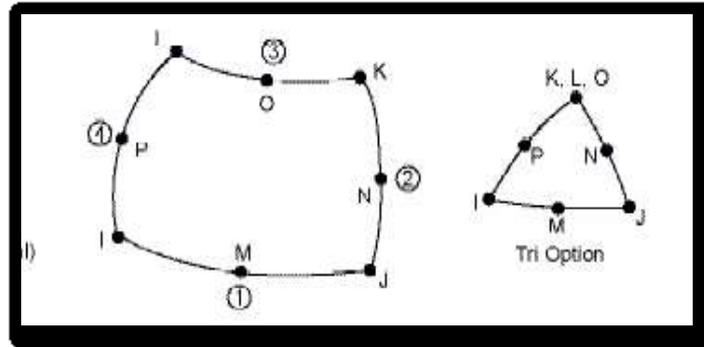
Figure (3): Element 183 geometry
