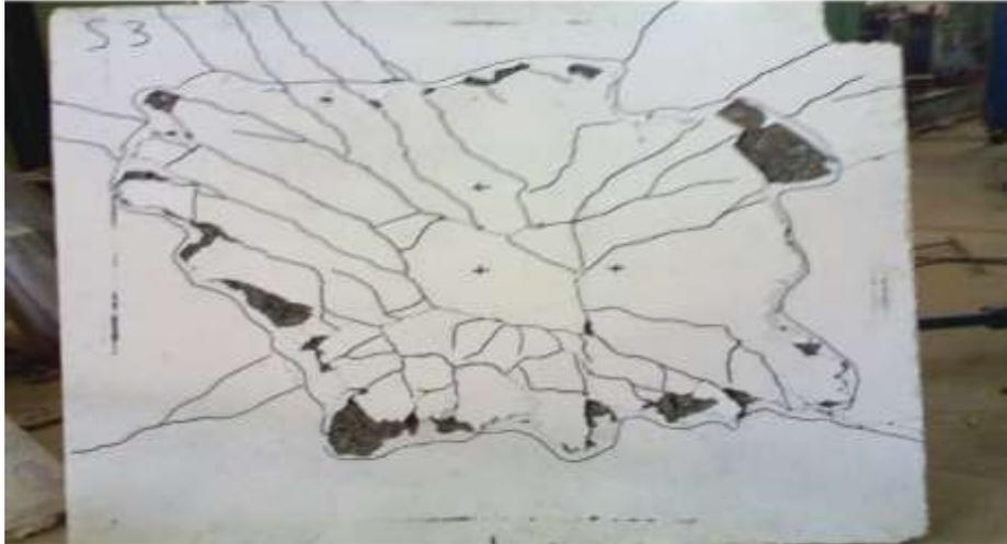
Figure (8) Crack patterns at tension face of slab S3
