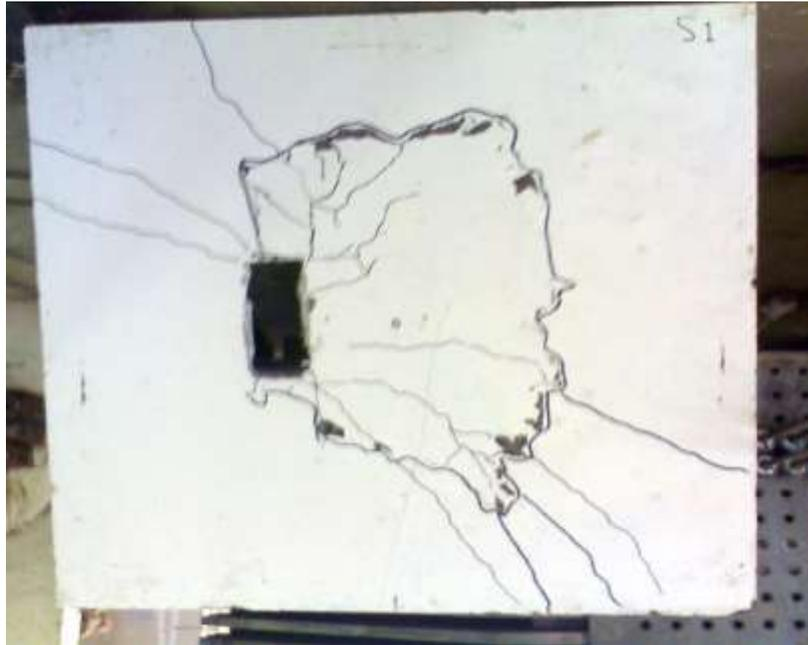
**Figure(6) Crack patterns at tension face of slab S1**
