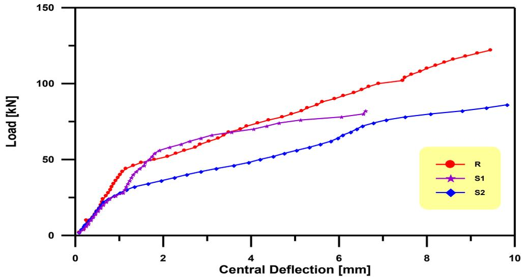
Figure(10) Load – central Deflection Curve for Slabs specimens R,S1 and S2
