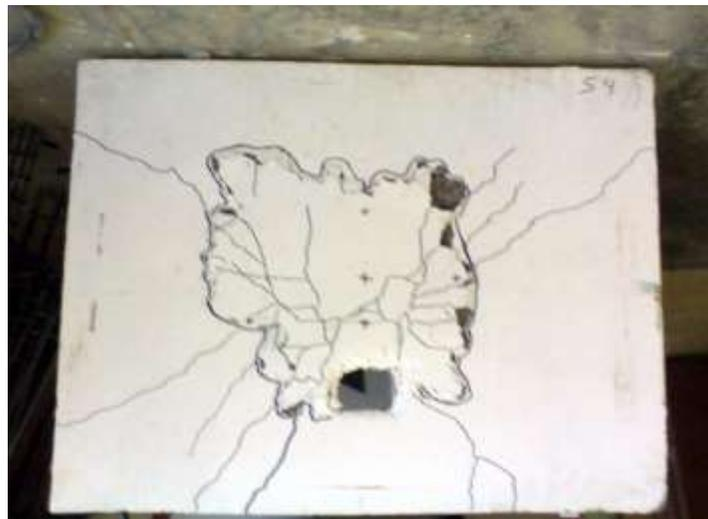
Figure(9) Crack patterns at tension face of slab S4
