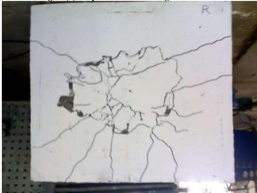
**Figure (5) Crack patterns at tension face of slab R**
