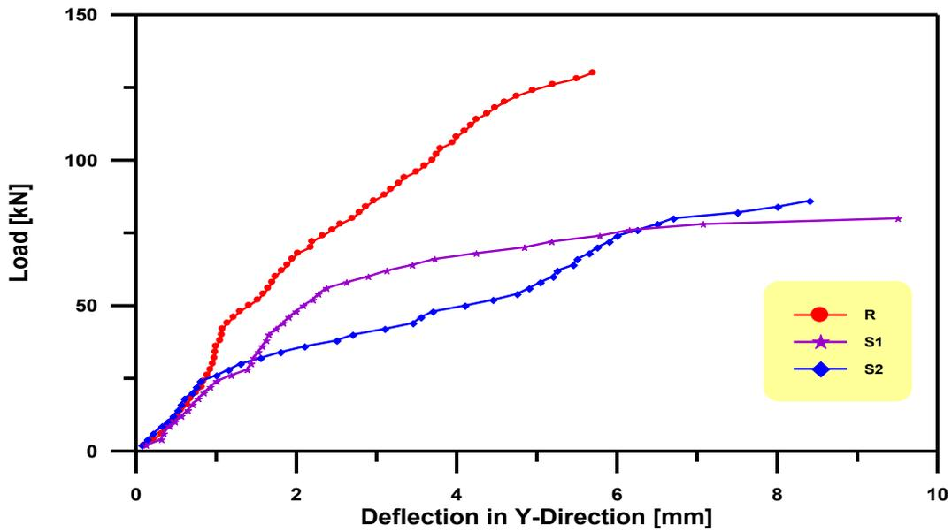
Figure(11) Load –Deflection Curve in Y-Direction for Slabs specimens R,S1 and S2
