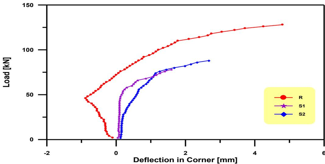
Figure(13) Load –Deflection Curve in Corner for Slabs specimens R,S1 and S2
