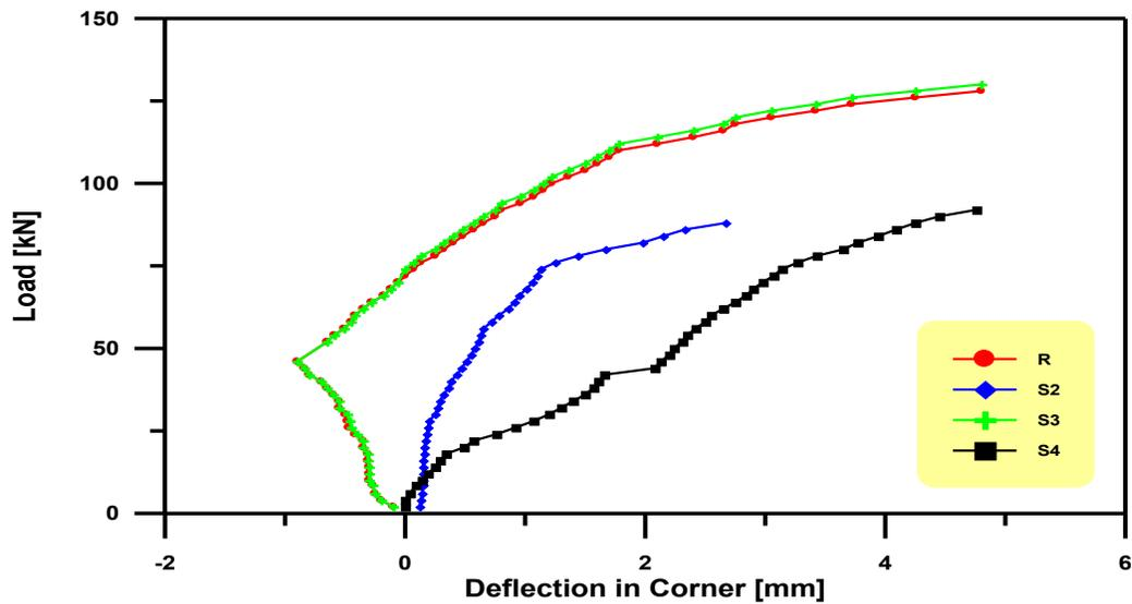
Figure (17) Load –Deflection in Corner Curve for Slabs specimens R,S2,S3 and S4
