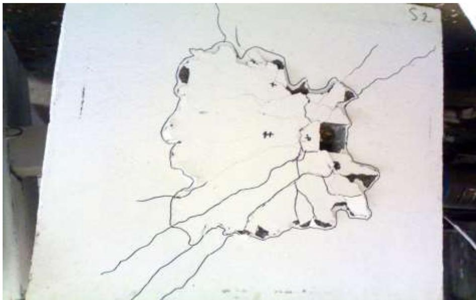
**Figure (7) Crack patterns at tension face of slab S2**
