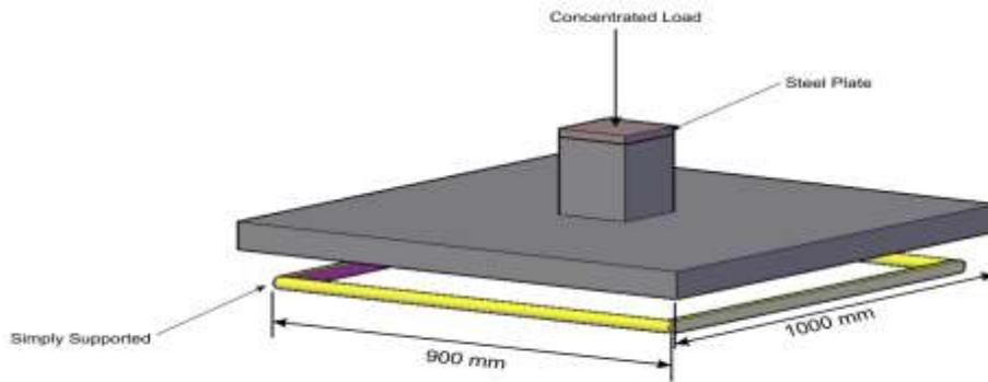
Figure(3) Loading and supporting of the slab
