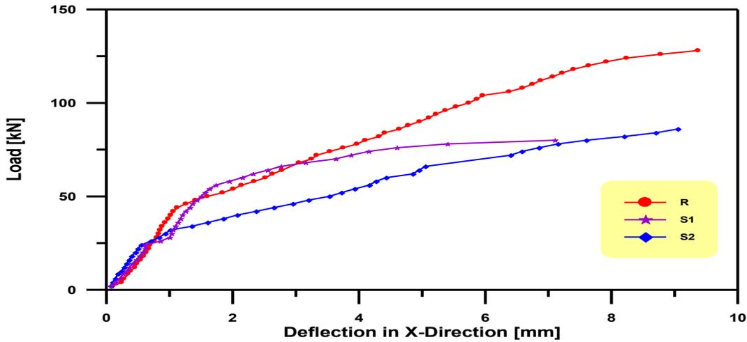
Figure(12) Load –Deflection Curve in X-Direction for Slabs specimens R,S1 and S2
