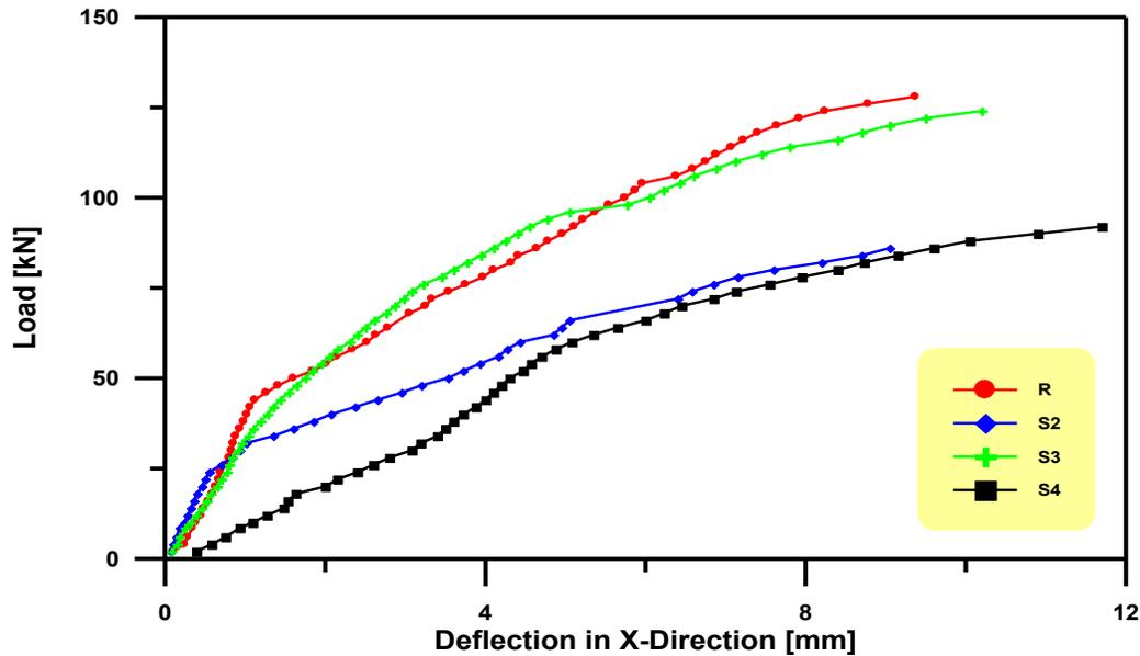
Figure.16 Load –Deflection in X-Direction Curve for Slabs specimens R,S2,S3 and S4
