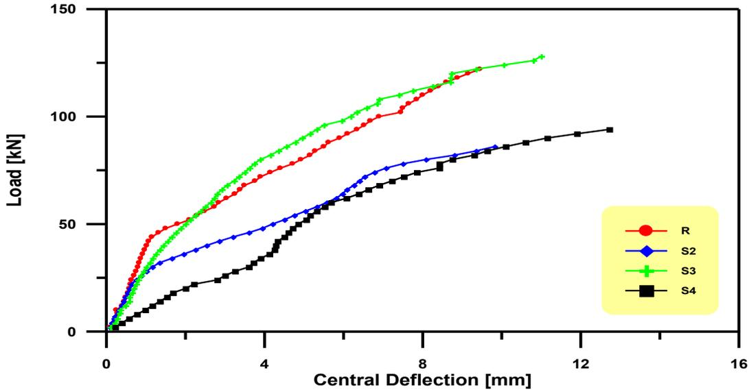
Figure(14) Load – central Deflection Curve for Slabs specimens R,S2,S3 and S4
