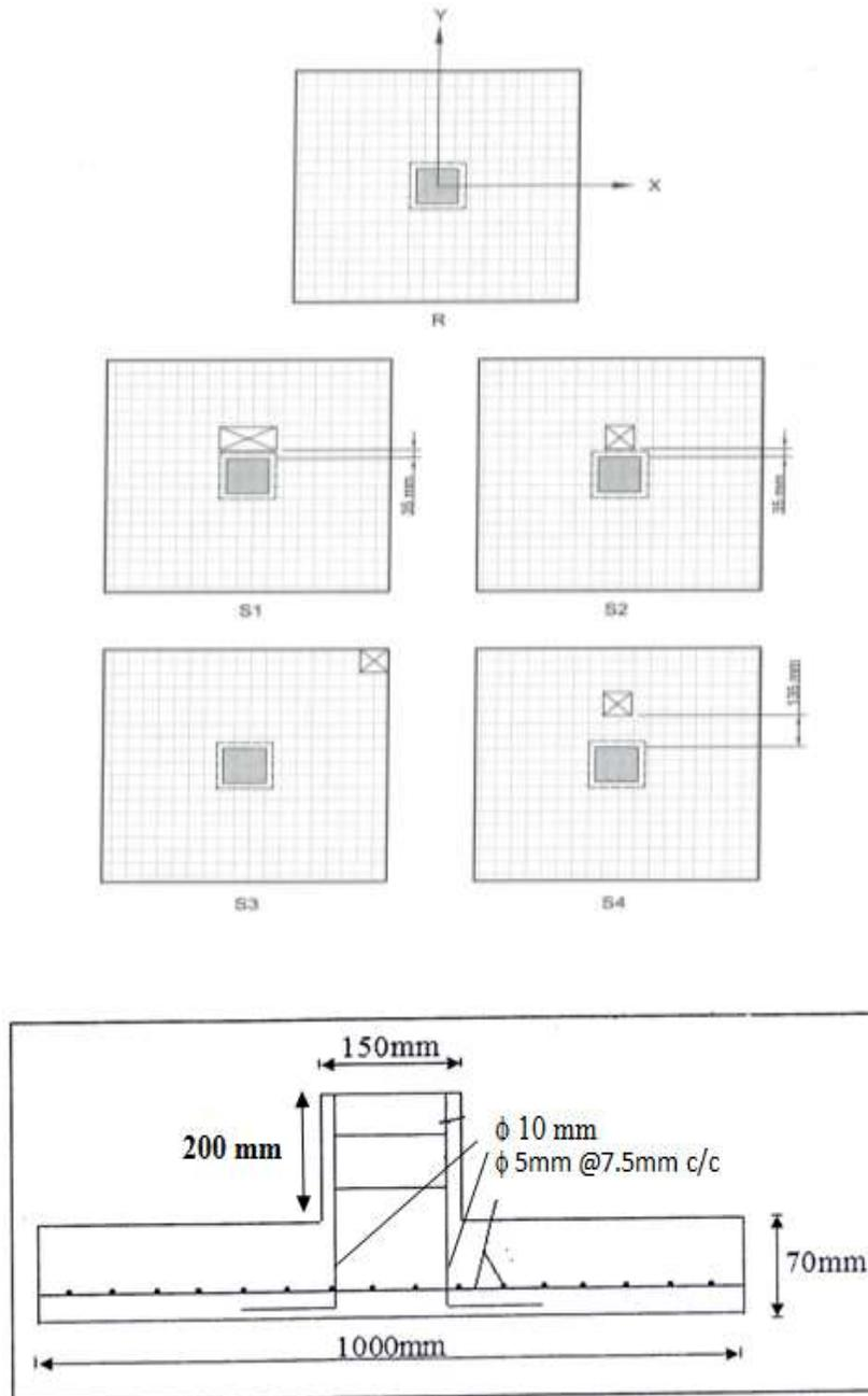
Figure(1) Model Slab With Location of Operation
