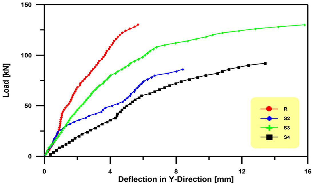
Figure(15) Load –Deflection in Y-Direction Curve for Slabs specimens R,S2,S3 and S4
