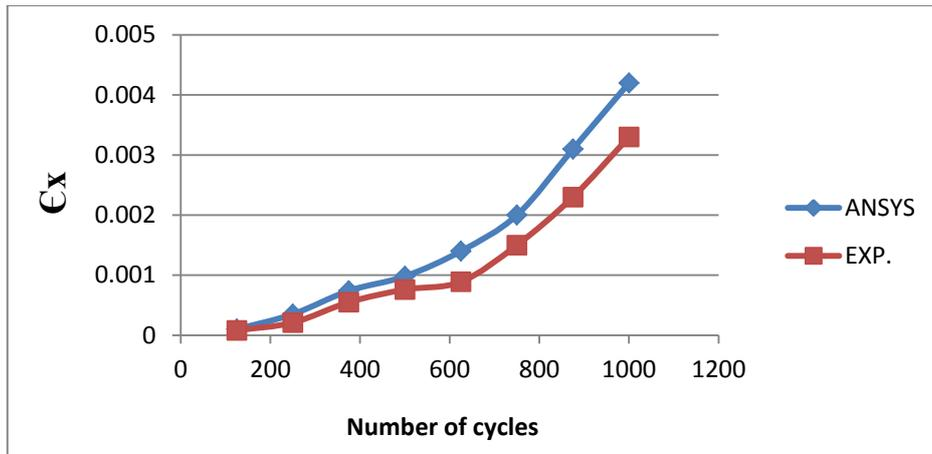
Figure (17).  $\epsilon_x$  numerical and experimental with number of cycles (AR=1.33,  $L_c=10\text{mm}$  & CSCS for Al-2024)
