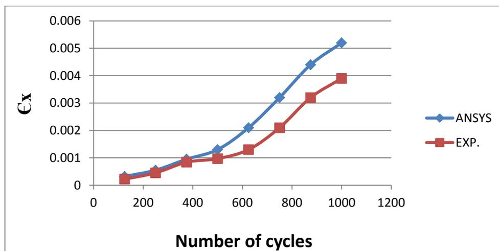
**Figure (13).**  $\epsilon_x$  numerical and experimental with number of cycles (AR=1.33, Lc=10mm & CSCS for Al-6061)
