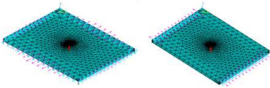
Figure (6). Loading and B.C.
