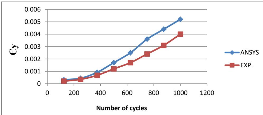
Figure (18).  $\epsilon_y$  numerical and experimental with number of cycles (AR=1.33,  $L_c=10\text{mm}$  & CSCS for Al-2024)
