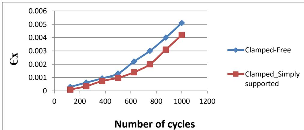
**Figure(21).  $C_x$  numerical with number of cycles (B.C: AR=1, Lc=12mm for Al- 2024)**
