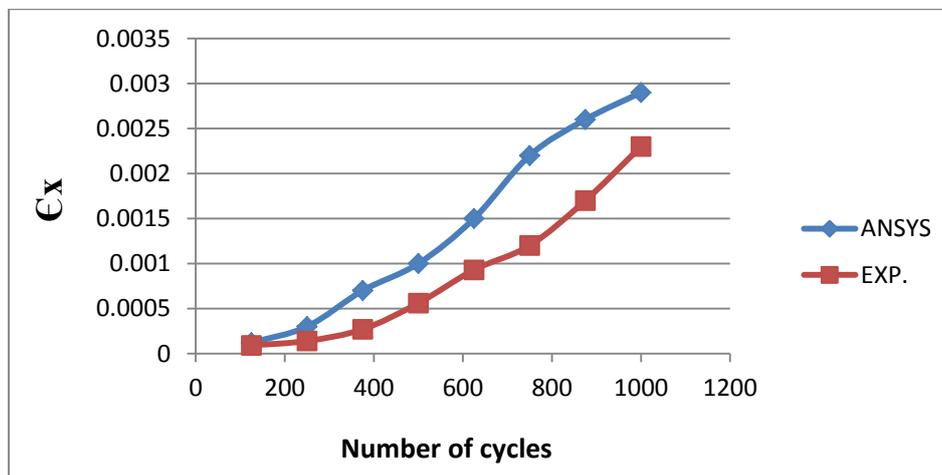
**Figure (15).**  $\epsilon_x$  numerical and experimental with number of cycles (AR=1.33,  $L_c=7\text{mm}$  & CSCS for Al-2024)
