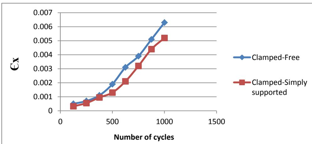
Figure (19).  $\epsilon_x$  numerical with number of cycles (B.C: AR=1,  $L_c=12\text{mm}$  for Al-6061)
