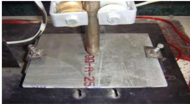
Figure (10). CFCF-boundary condition
