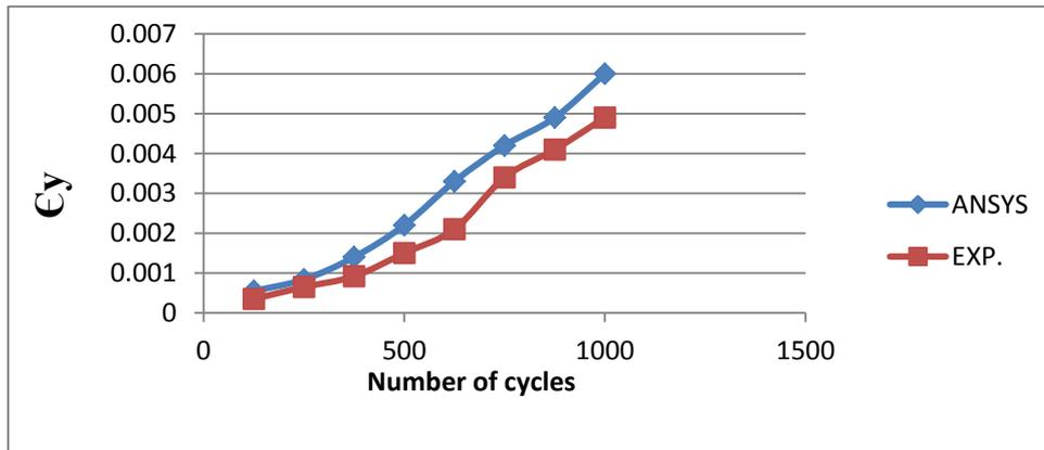
**Figure (14).**  $\epsilon_y$  numerical and experimental with number of cycles (AR=1.33,  $L_c=10\text{mm}$  & CSCS for Al-6061)
