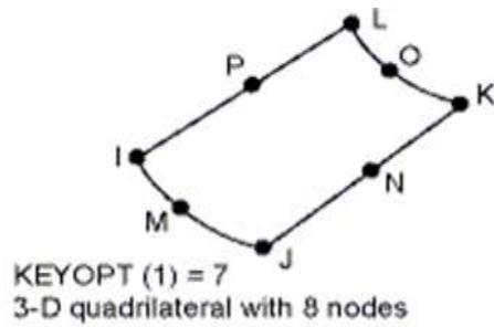
**Figure (2). Mesh200 Element Geometry.**
