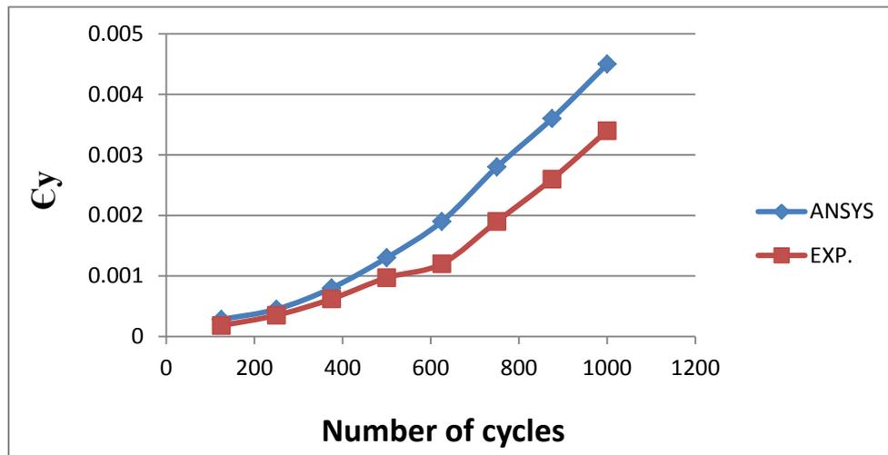
**Figure (12).**  $\epsilon_y$  numerical and experimental with number of cycles (AR=1.33, Lc=7mm & CSCS for Al-6061)
