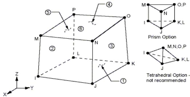
**Figure (1). Solid185 element geometry.**
