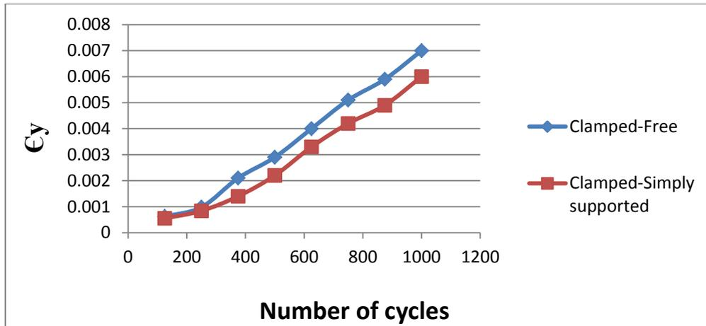
**Figure (20).  $C_y$  numerical with number of cycles (B.C: AR=1, Lc=12mm for Al-6061)**
