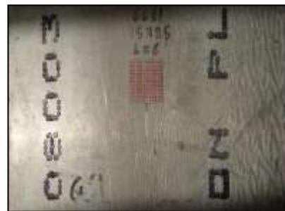
**Figure (4). A printed grid on the plate (Al-6061)**
