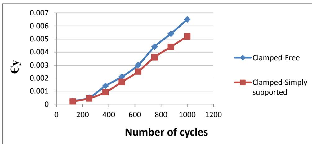
**Figure(22).  $C_y$  numerical with number of cycles (B.C: AR=1, Lc=12mm for Al-2024)**
