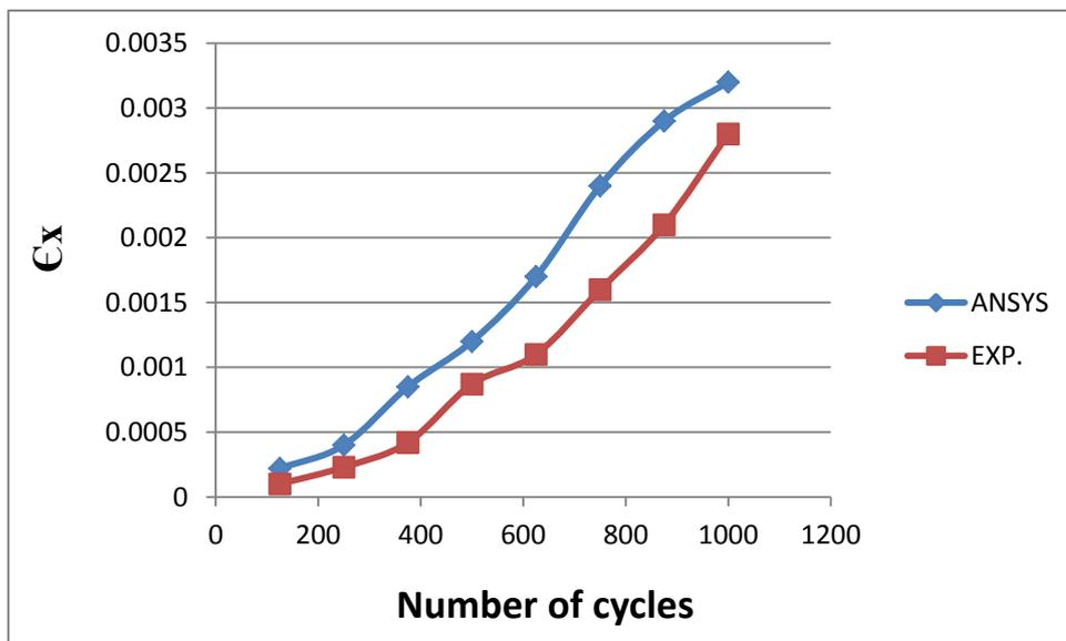
Figure (11).  $\epsilon_x$  numerical and experimental with number of cycles (AR=1.33,  $L_c=7\text{mm}$  & CSCS for Al-6061)
