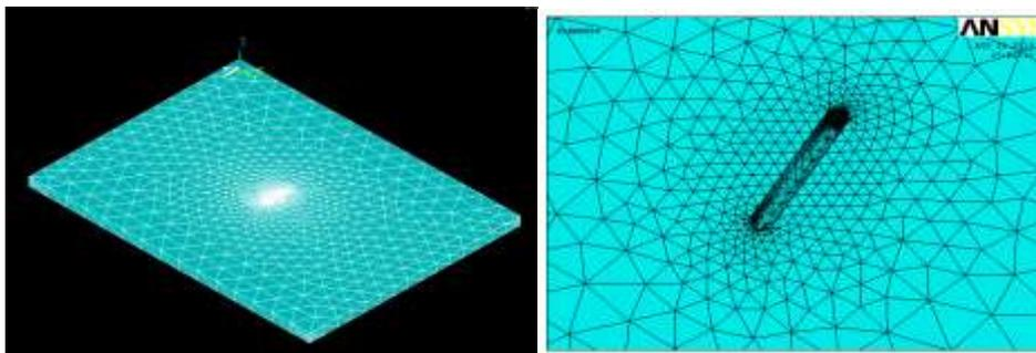
**Figure(5). 3D Model with solid185.**
