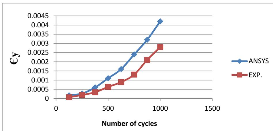
**Figure (16).**  $\epsilon_y$  numerical and experimental with number of cycles (AR=1.33,  $L_c=7\text{mm}$  & CSCS for Al-2024)
