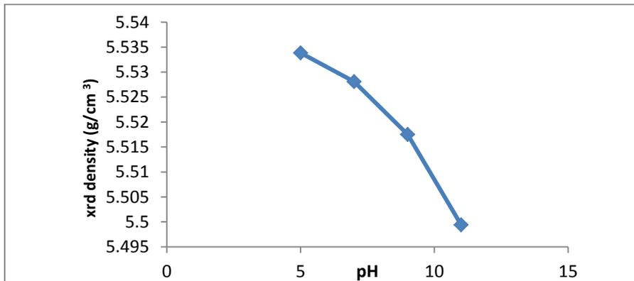
Figure (4): Plot of XRD density as a factor of pH, for powders at 500°C.
