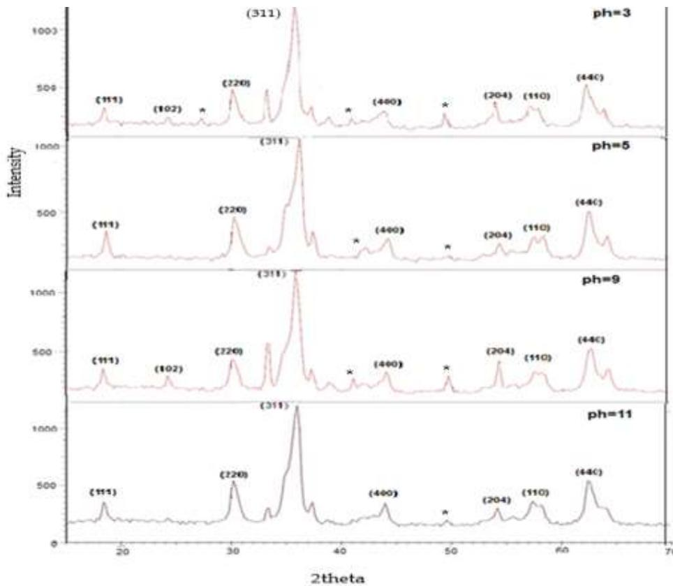
Figure (1): XRD patrons of samples with deferent pH, show that all peaks indexed to pure cubic phase, with extra peak denote by (\*)of CuO, and Fe<sub>2</sub>O<sub>3</sub>
