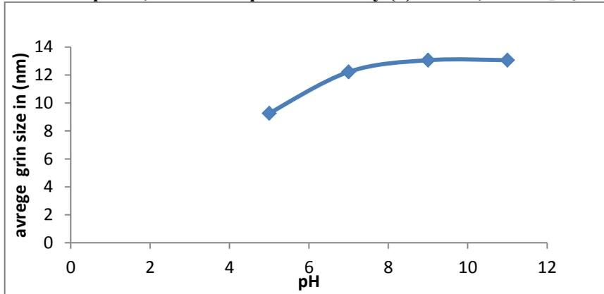
Figure (2): Plot of average grin size of samples as a factor of pH denotes an increase of average grain size with increasing pH value.
