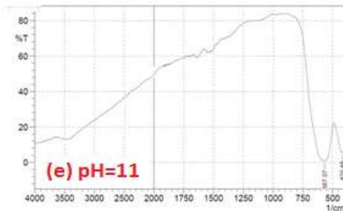
**Figure (9a,b,c,d,e): FTIR patron of samples with different pH show that formation of spinel structure with two main absorption band  $V_1$  and  $V_2$  as common feature of FTIR in the rang of  $(2000-500) \text{ cm}^{-1}$**
