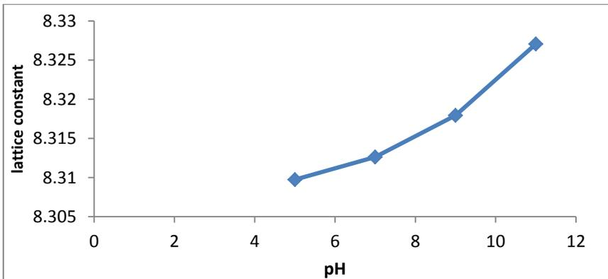
Figure (3): Plot of lattice constant as a factor of pH, for powders at 500°C
