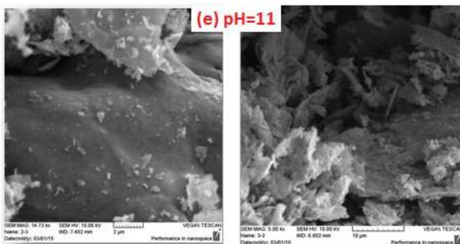
Figure (4,a,b,c,d,e): SEM images of  $\text{CuFe}_2\text{O}_4$  samples after calcination  $500^\circ\text{C}$  present porosity and boundary between neighboring particles can also be observed
