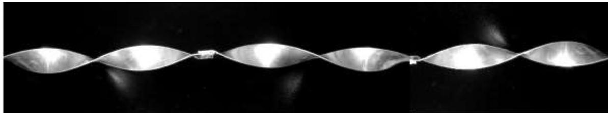
Figure (4) Clockwise - counter clockwise twisted tape
