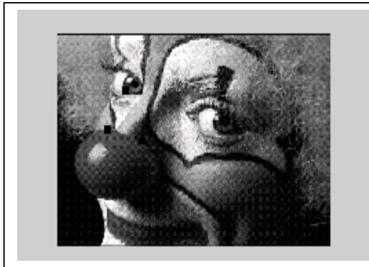
Fig.(4) The Simulated Lost Blocks. The Black Squares Represent The Lost Blocks
