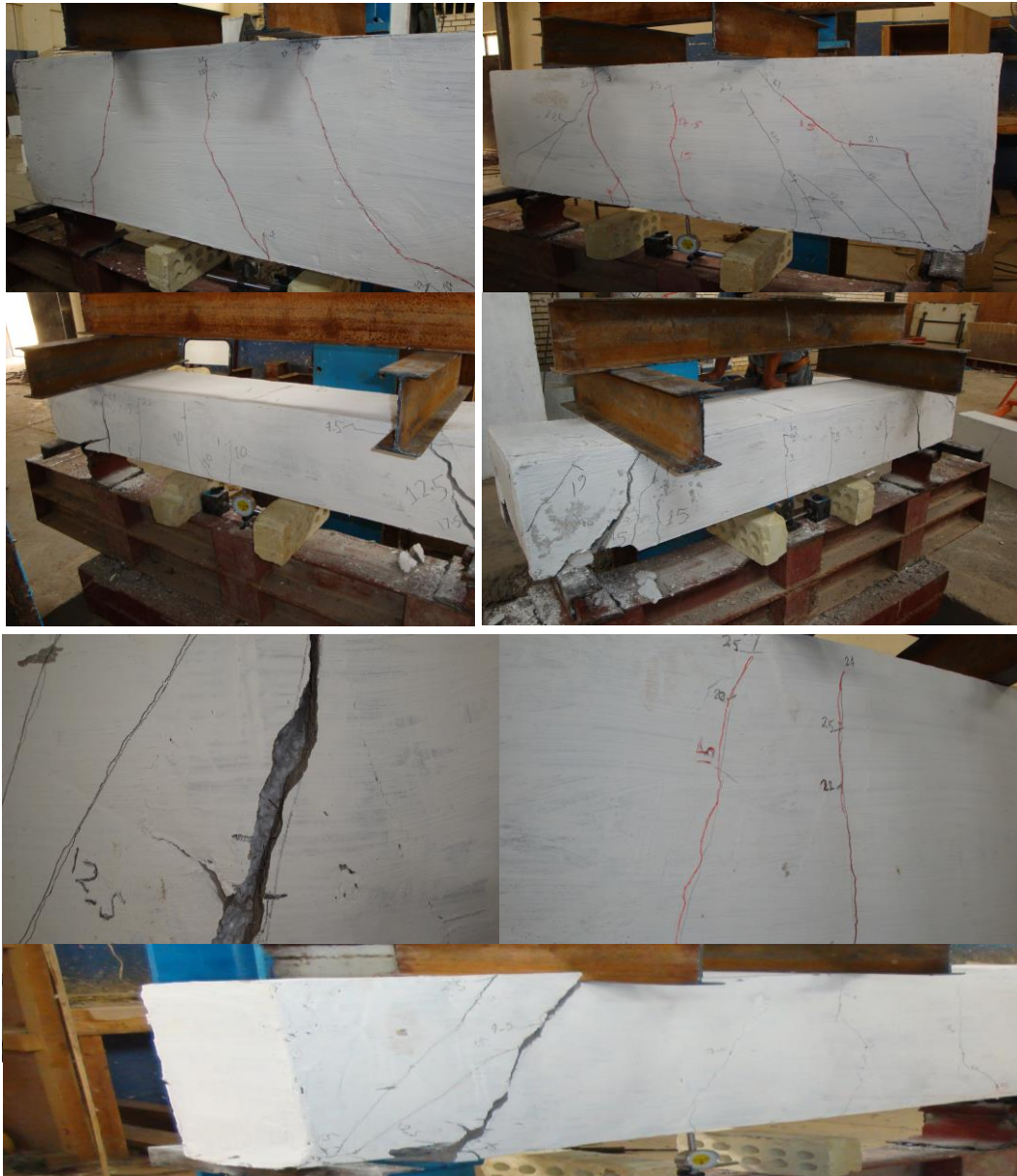
Fig.(6) Crack pattern for Monopanel beam specimens
