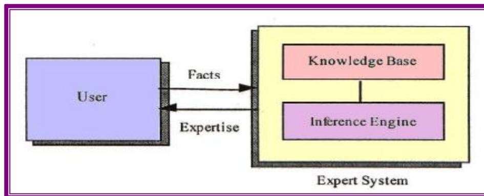
Figure 1. Represent of basic concept of an expert system
