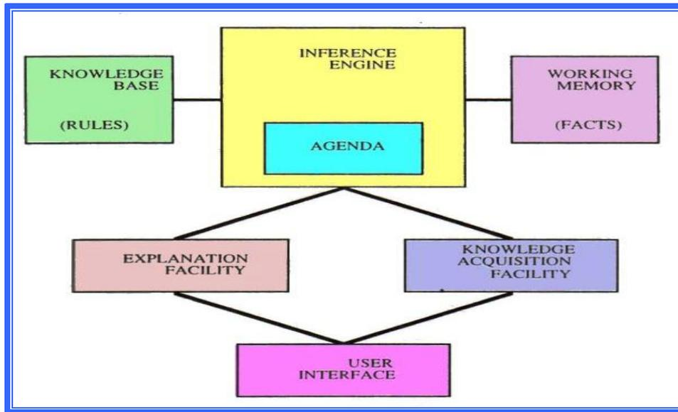
Figure 3. Structure of a Rule based expert system
