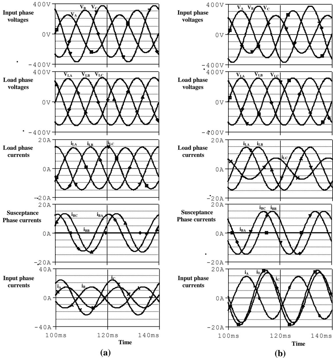
**Fig. 14** Voltage and current waveforms during random changes in input phase voltages when the regulator was (a) fully loaded by balanced 0.8 power factor inductive impedance, (b) randomly loaded.
