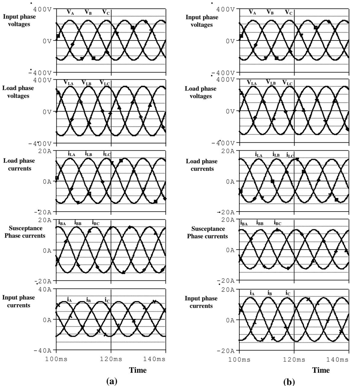
**Fig. 12 Regulator voltage and current waveforms during a drop in each input phase voltage of 20% of its rated value at full-load operation with balanced three-phase (a) pure resistive load, (b) inductive load running at 0.8 power factor.**
