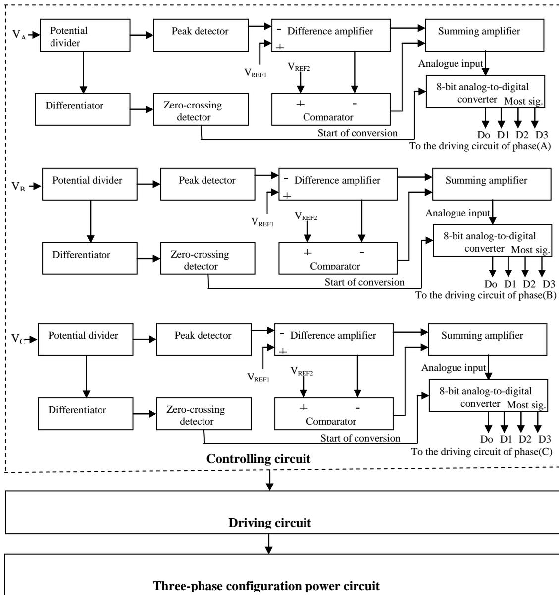
Fig. 6 The proposed three-phase regulator schematic design.
