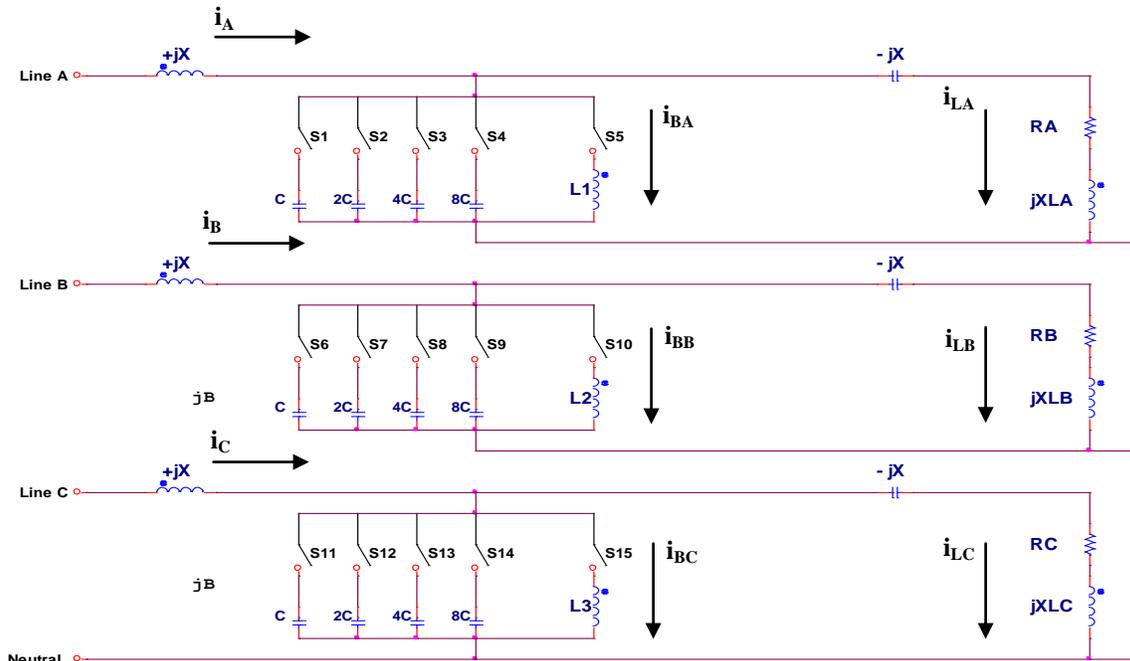
Fig. 5 Three-phase configuration of the proposed regulator.
