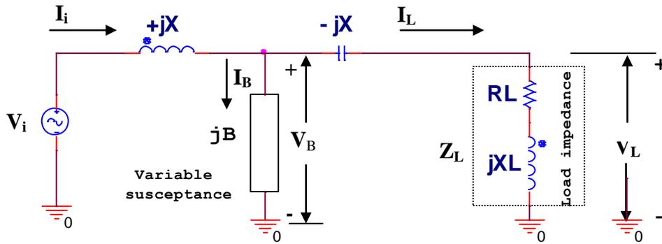
**Fig. 1** Single-phase circuit of the proposed regulator.
