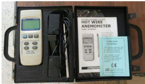
Figure (6) Hot Wire Anemometer
