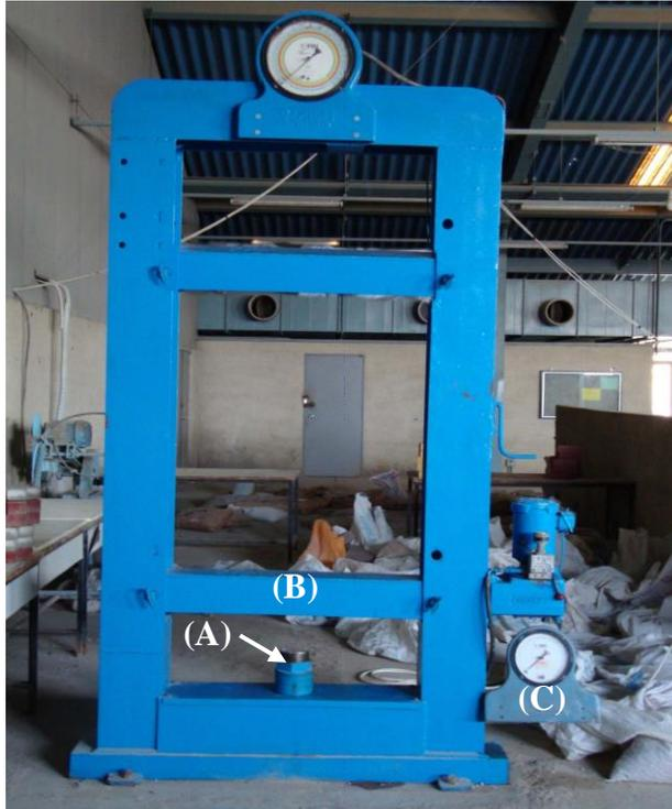
(A) The load cell unit with 1500kN capacity
