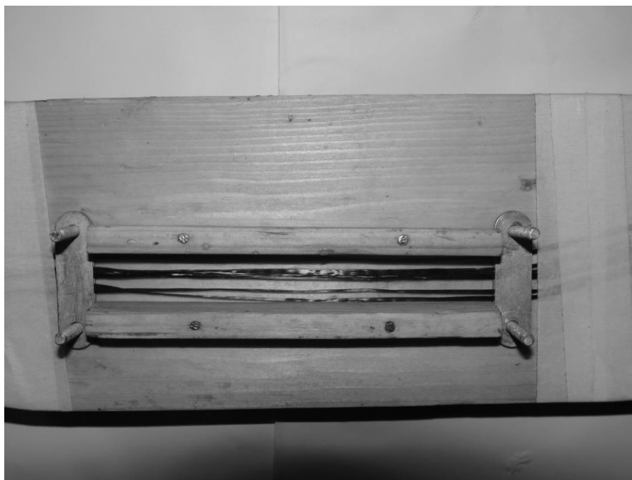
Fig. 1: Flexural sample mold for composite materials
