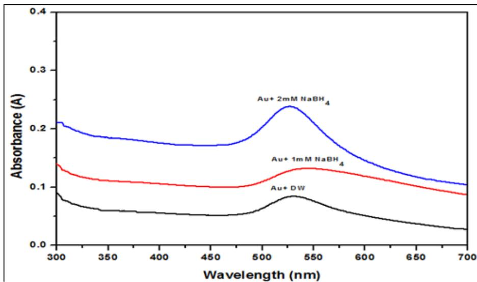
**Fig. (2): UV-Visible absorption spectra of colloidal gold nanoparticles.**
