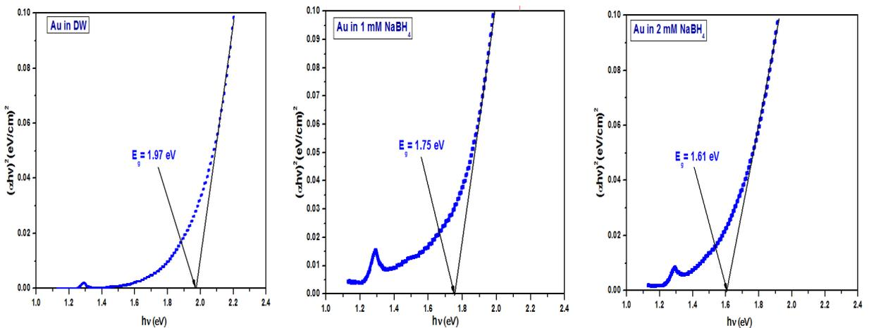
**Fig. (3): Colloidal gold nanoparticle samples' direct band gap calculations.**
