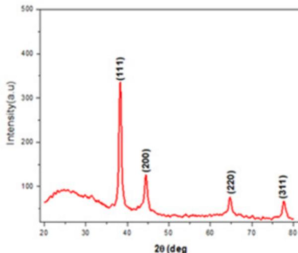
Figure 1. XRD patterns of Au NPs.
