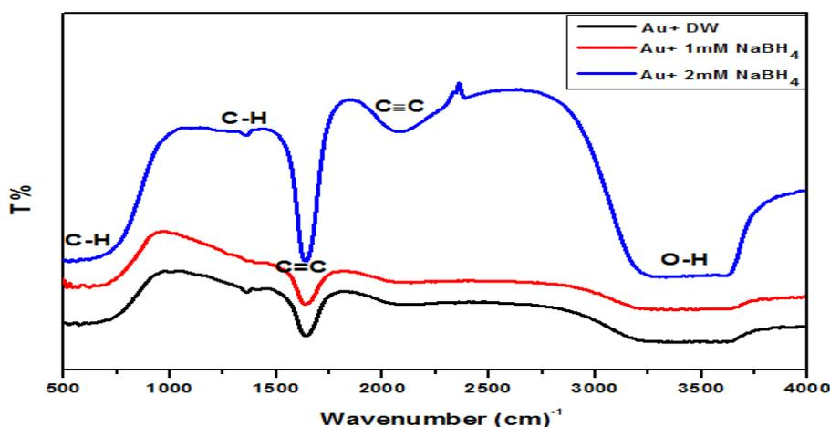
**Fig.(4): FTIR spectrums of gold nanoparticle prepared in solutions (DW, 1mM NaBH<sub>4</sub>, 2mM NaBH<sub>4</sub>)**
