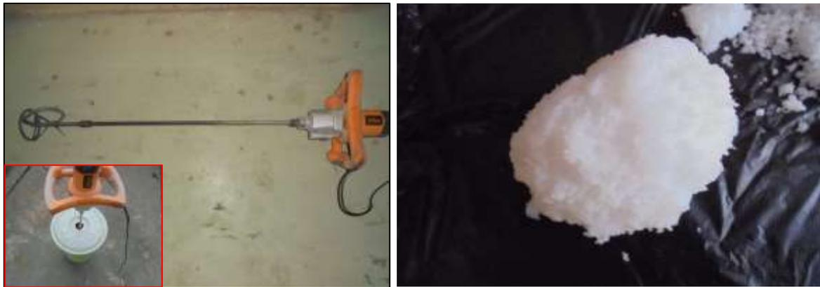
**Figure (2):- Left: mixer used in dry mixing of nano silica; and right: nano silica agglomeration after mixing with water in a ratio of 15: 85 (nano silica: water).**
