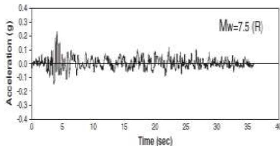
Figure (5). Far field acceleration record of Hachinohe earthquake (1968).
