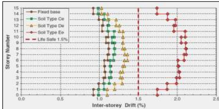
Figure 7. Elastic inter-storey drifts for model S15 resting on soil classes  $C_e$ ,  $D_e$  and  $E_e$  with bedrock depth of 30 m.
