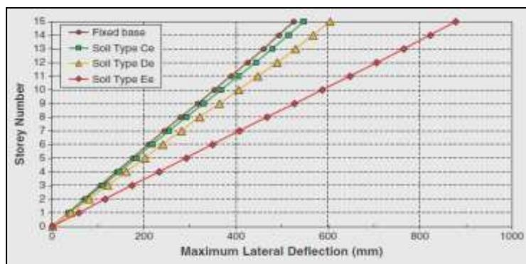
Figure 8. Inelastic storey deflections for model S15 resting on soil classes  $C_e$ ,  $D_e$  and  $E_e$  with bedrock depth of 30 m.
