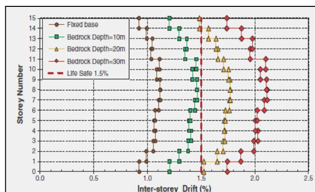
Figure (10). Elastic inter-storey drifts for model S15 resting on soil class  $E_e$  with variable bedrock depths.
