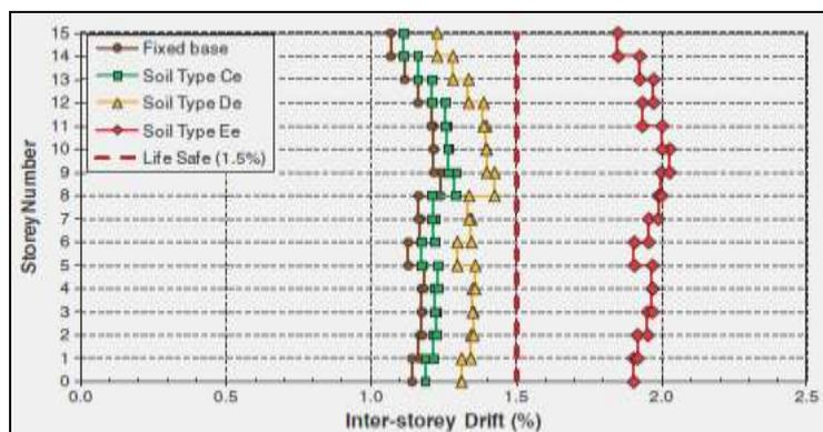
Figure 9. Inelastic inter-storey drifts for model S15 resting on soil classes  $C_e$ ,  $D_e$  and  $E_e$  with bedrock depth of 30 m.
