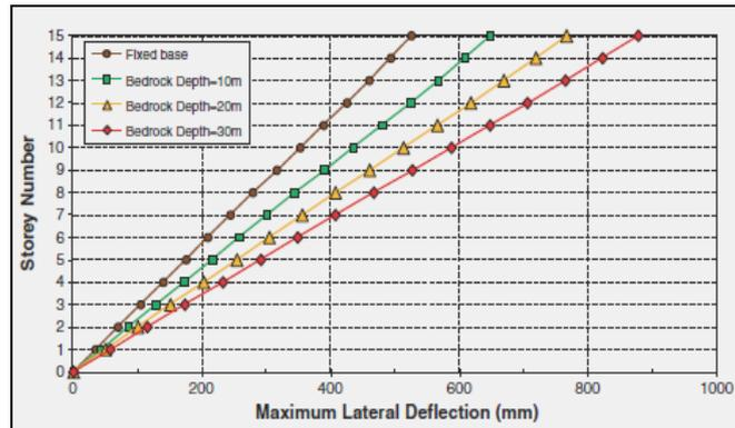
Figure (11). Inelastic storey deflections for model S15 resting on soil class Ee with variable bedrock depths.
