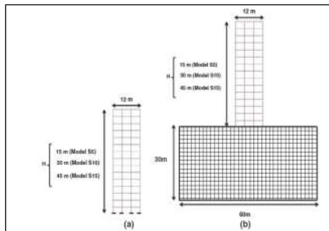
**Figure (1). Numerical models: (a) fixed base model; (b) flexible base model.**
