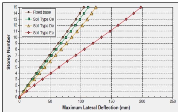
**Figure (6). Elastic storey deflections for model S15 resting on soil classes C<sub>e</sub>, D<sub>e</sub> and E<sub>e</sub> with bedrock depth of 30 m.**
