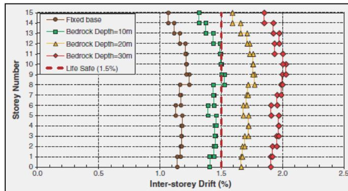
Figure (12). Inelastic inter-storey drifts for model S15 resting on soil class Ee with variable bedrock depths.
