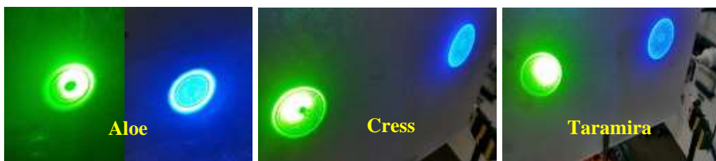
Fig(4): Rings appeared in Aloe oil , Cresson oil and Taramira oil using blue and green lights at the same time
