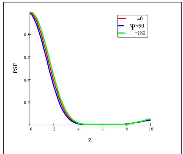
Figure (3)PSF for four apertures with coma aberration (0.25) and different values of rotation angle coefficient.(R=1,ε=0.75).
