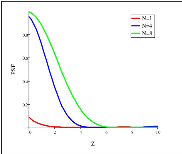
Figure (4)PSF for rotation angle (45) with obscuration ratio (0.25) and different values number of apertures.(R=1,w<sub>31</sub>=0.75).
