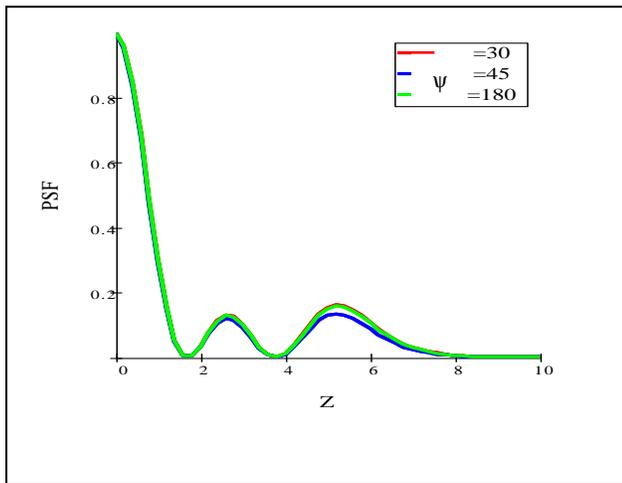
Figure (5)PSF for eight apertures with no obscuration and different values of rotation angle coefficient .(w<sub>31</sub>=0.5,R=4).
