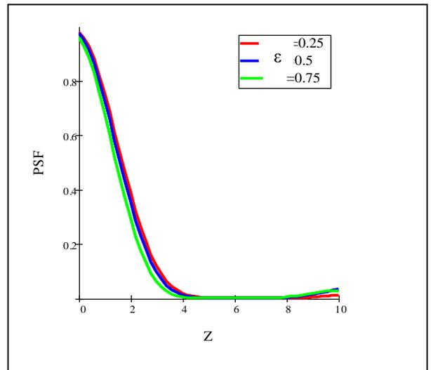
Figure (2)PSF for four apertures with coma aberration (0.5) and different values of obscuration ratio coefficient (R=1,ψ=90).
