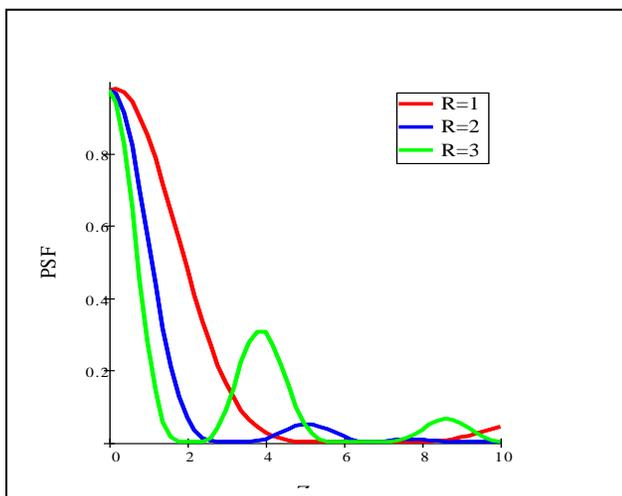
Figure(6)PSF for four apertures with obscuration ratio (0.5) and different values of distance coefficient.(w<sub>31</sub>=0.5,ψ=180).
