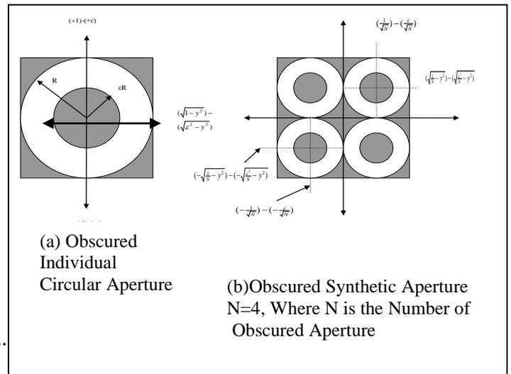
Figure (1) The Integral Boundary for Array of Obscured Circular Synthetic Aperture
