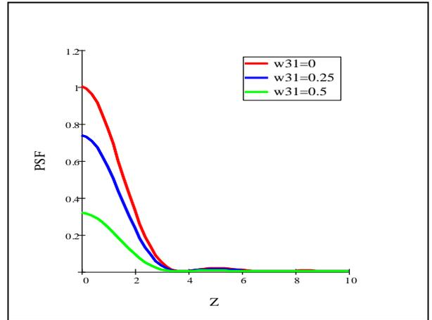
Figure (1)PSF for individual aperture with no obscuration and different values of coma aberration.
