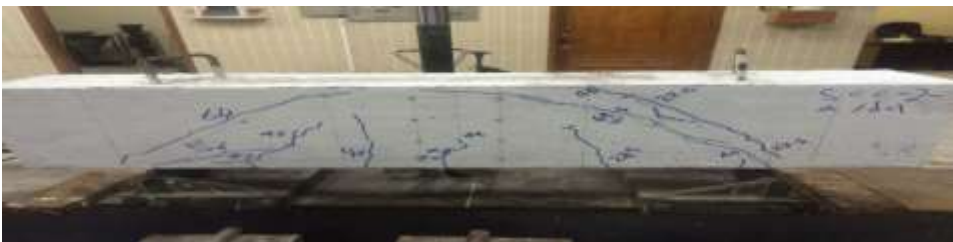
Fig. (5): Crack Pattern for Beam A-1
