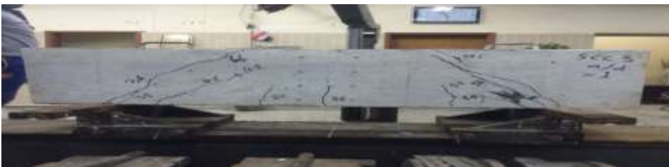
Fig. (7): Crack Pattern for Beam C-1
