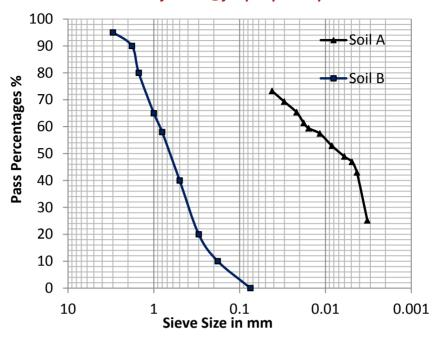
Figure 1: Grain Size Distribution of Soil A and Soil B
