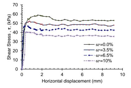
Figure 6: Relationship between shear stress versus horizontal displacement at  $(\sigma n) = 100 \text{ kPa}$
