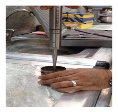
Figure 3: Hand vane shear tester
