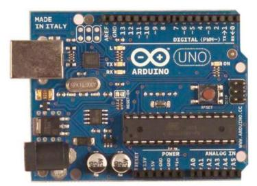
Figure (4): Arduino Uno microcontroller board
