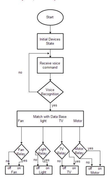
Figure (11): Flowchart for system algorithm
