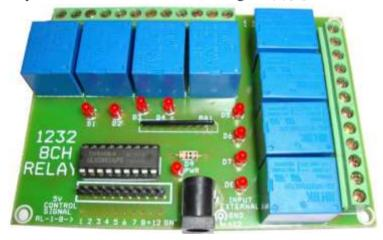
Figure (6): Relay Board – 8 Channels
