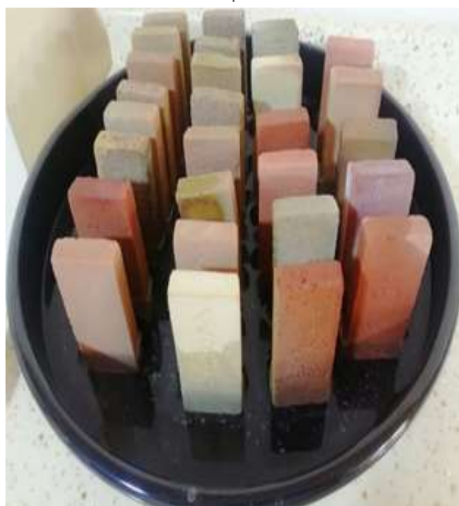
Figure. 5. Brick samples of Al-Angor with different ratios of BaCO 3 .
