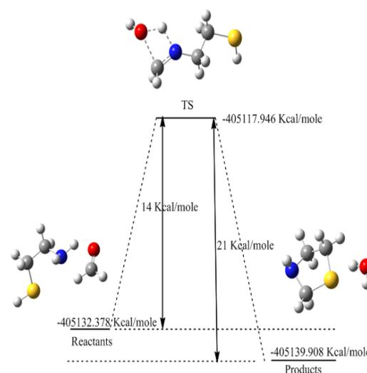
Fig. 3 The Geometry of TS12 Transition state structures of Formaldehyde with 2-aminoethanthiol from IRC Calculation at RHF/6-31++g(2d,2p).
