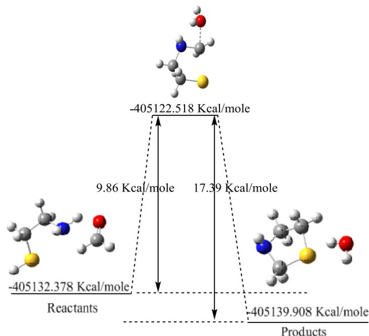
Fig. 6 Thiazolidine formation reaction at UHF/6-31++G (2d, 2p) according to scheme 2.
