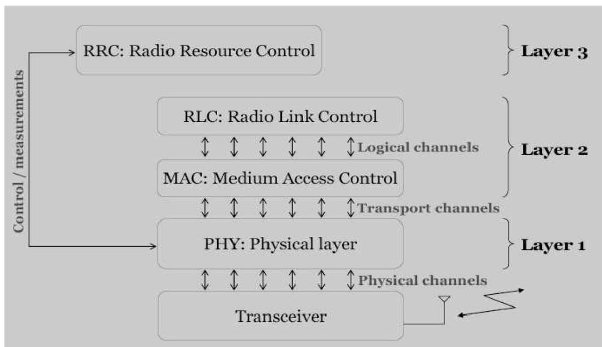
Figure 3 - LTE protocol Architecture.
