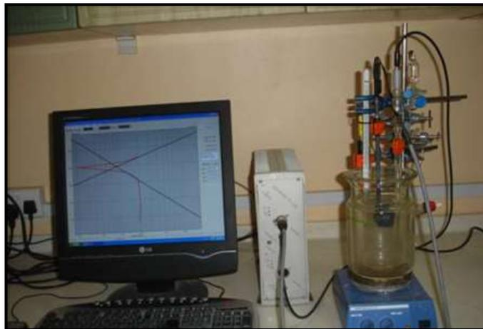
Figure (1).Potentiostat (Wenking LT87-Germany)
