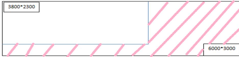
Figure (8). Preparation Using 6000\*3000mm Plates
