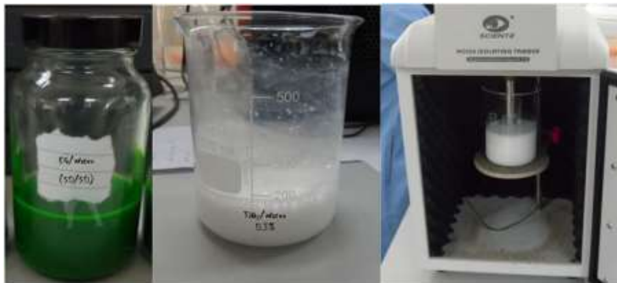
Figure(2) Ethylene glycol/water (50/50) and (0.3% TiO 2 /water) nanofluid samples with ultrasonic homogenizer
