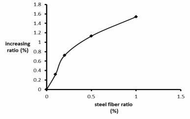
Figure (2): Increasing of tensile strength with various steel fiber ratio.
