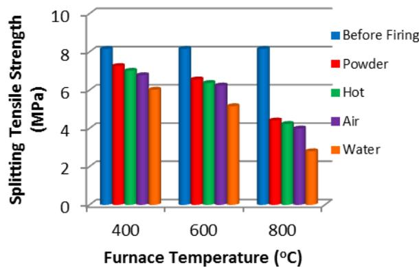
Figure (8) Splitting Tensile Strength for (DF3NMC80) before and after exposure to fire flame temperature with different cooling for (1)Hour
