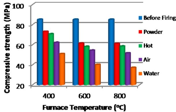
Figure (3) Compressive Strength of (GF3NMC801) before and after exposure to fire flame temperature with different cooling for (1.5)Hour
