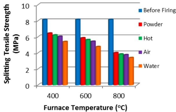
Figure (10) Splitting Tensile Strength for (DF3NMC80<sub>1</sub>) before and after exposure to fire flame temperature with different cooling for (1.5)Hour
