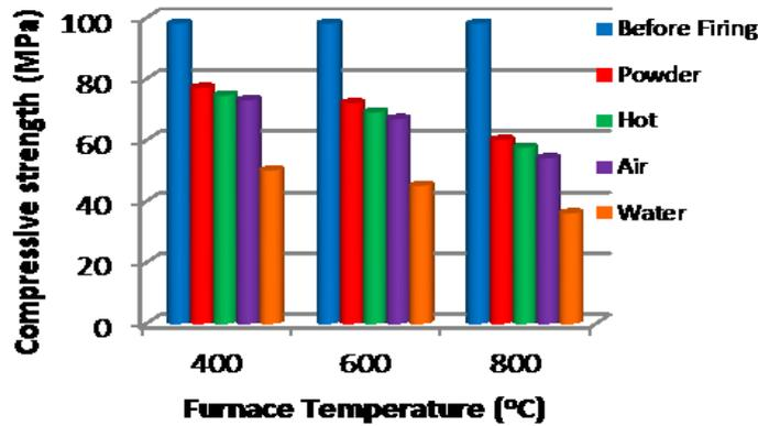
Figure (6) Compressive Strength of (D5NMC80) before and after exposure to fire flame temperature with different cooling for (2)Hour
