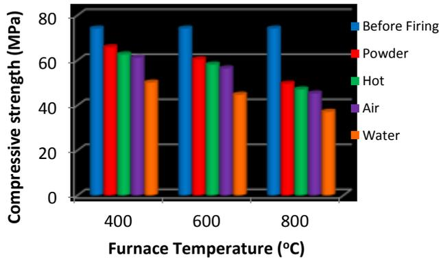
Figure (4) Compressive Strength of (D5NMC802) before and after exposure to fire flame temperature with different cooling for (1.5)Hour
