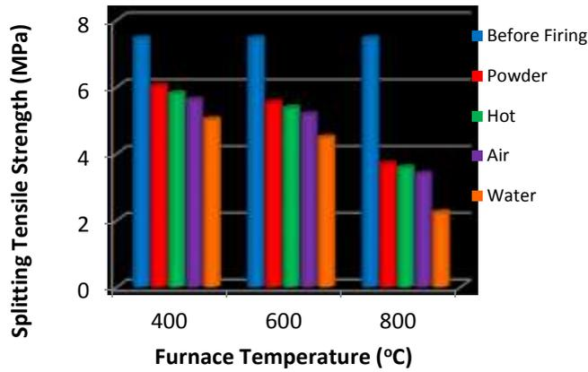
Figure (12) Splitting Tensile Strength for (DF3NMC80<sub>1</sub>) before and after exposure to fire flame temperature with different cooling for (2)Hour
