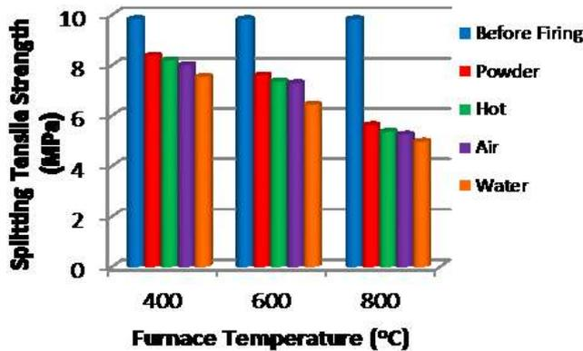
Figure (7) Splitting Tensile Strength for (G5NMC80) before and after exposure to fire flame temperature with different cooling for (1)Hour
