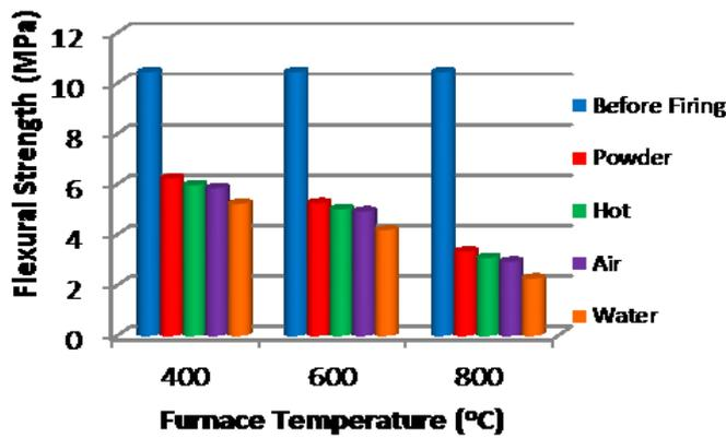
Figure (13) Flexural Strength of (G5NMC80<sub>2</sub>) before and after exposure to fire flame temperature with different cooling for (1)Hour
