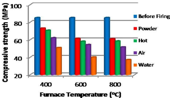
Figure (5) Compressive Strength of (GF3NMC801) before and after exposure to fire flame temperature with different cooling for (2)Hour
