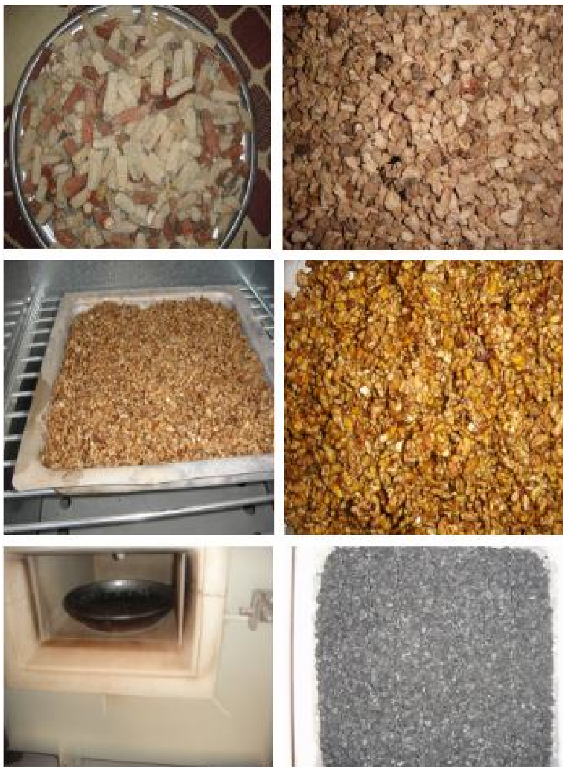
Fig. (2) The Steps of Corncob Activated Carbon Preparation
