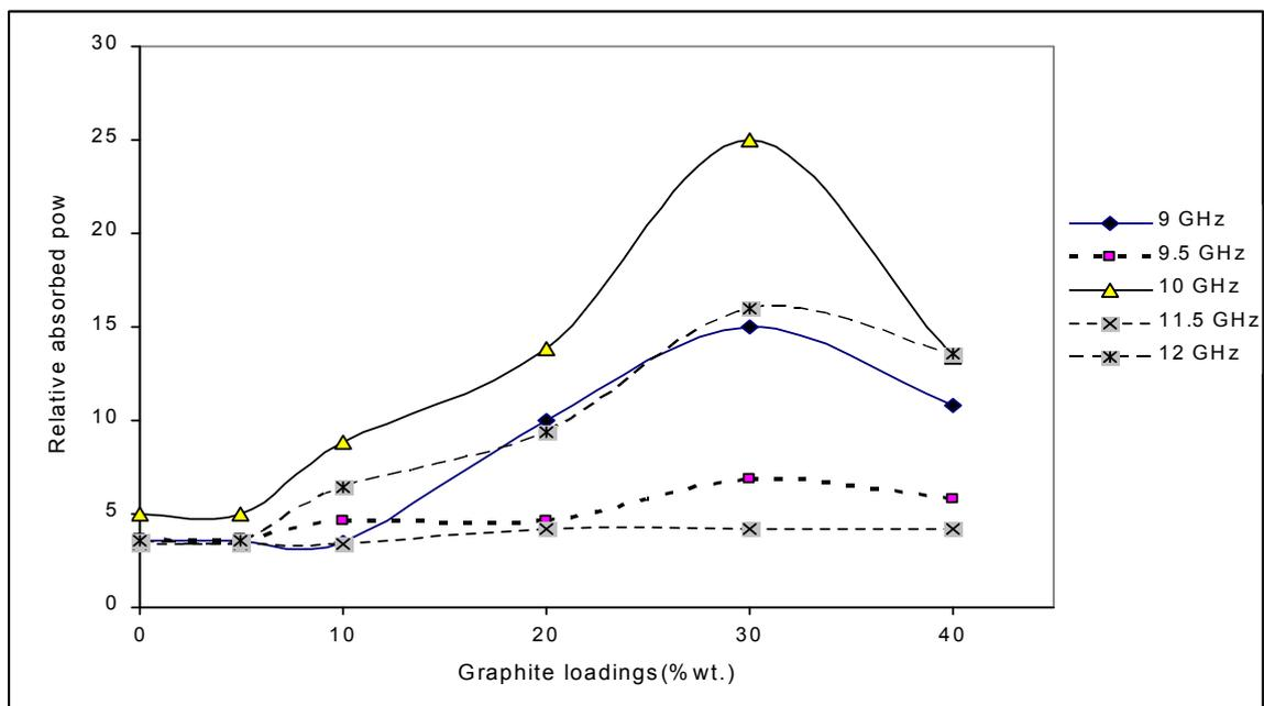
**Fig (5): The variation of relative absorbed power as a function of graphite loading in (SPUF/Gr) composites.**
