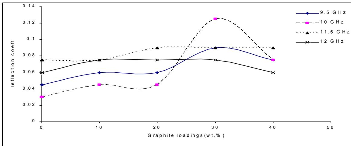
**Fig (3):** The variation of reflection coefficient as a function of graphite loadings in (SPUF/Gr) composites.
