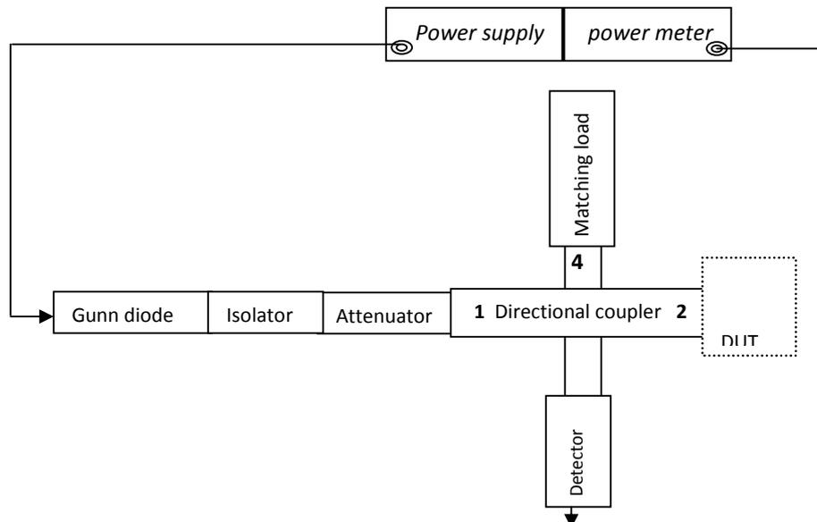
Fig. 1: Experimental setup for measurement
