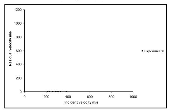
Fig.13. Final velocity V(r) versus incident velocity V(i) for 30 layer woven composite by hemispherical projectile
