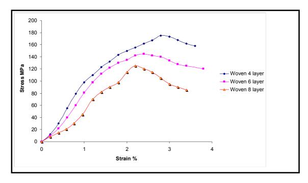
Fig. 4. Tensile stress strain for composite materials woven Kevlar
