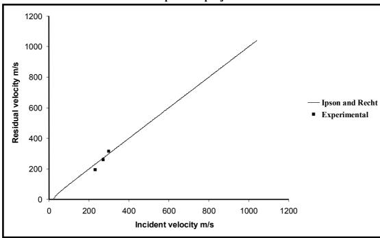
Fig. 7. Final velocity V(r) versus incident velocity V(i) for 3 layer woven composite by hemispherical projectile
