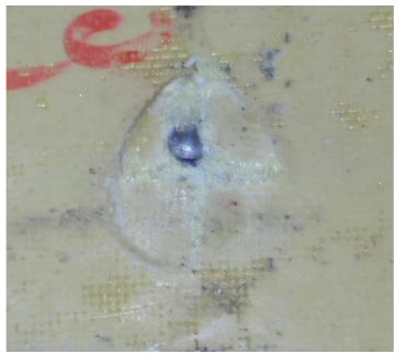
Fig.16. Composite material target of 30 layer woven fiber Kevlar/  $Al_2O_3$  powder in a Epoxy matrix struck by a hemispherical projectile as  $V_i = 390.87$  m/s
