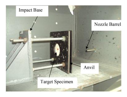
Fig. 2 The target specimen has been placed between the base and the anvil
