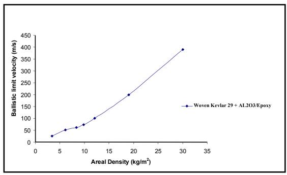
Fig. 6. Ballistic Performance of armor composite material versus areal density by hemispherical projectile
