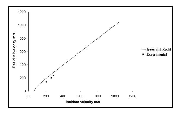
Fig. 10. Final velocity V(r) versus incident velocity V(i) for 8 layer woven composite by hemispherical projectile
