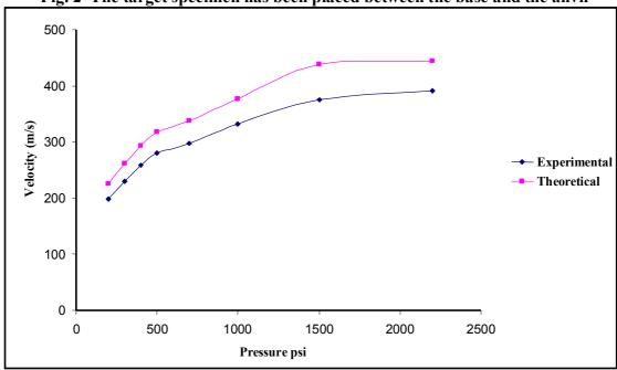
Fig. 3. Velocity measured with pressure for gas gun
