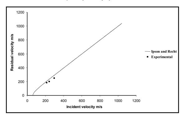
Fig. 9. Final velocity V(r) versus incident velocity V(i) for 6 layer woven composite by hemispherical projectile
