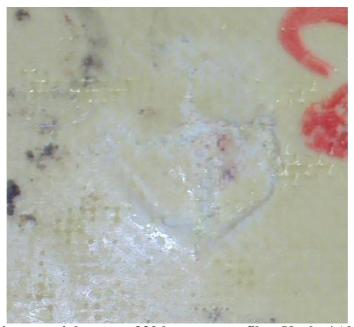
Fig.15. Composite material target of 30 layer woven fiber Kevlar/  $Al_2O_3$  powder in a Epoxy matrix struck by a hemispherical projectile as  $V_i = 385$  m/s
