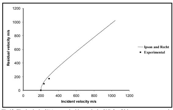
Fig.12. Final velocity V(r) versus incident velocity V(i) for 20 layer woven composite by hemispherical projectile
