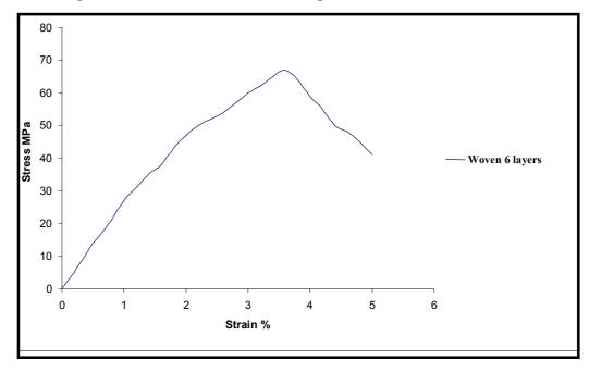
Fig 5. Compression stress strain for composite 6 layer woven Kevlar
