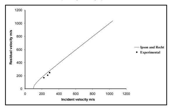
Fig. 11. Final velocity V(r) versus incident velocity V(i) for 10 layer woven composite by hemispherical projectile
