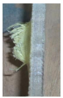
Fig.14. A cross sectional view of perforated zone composite material target of 20 layer woven fiber Kevlar/  $Al_2O_3$  powder in a Epoxy matrix struck by a hemispherical projectile as  $V_i$  = 321.78 m/s
