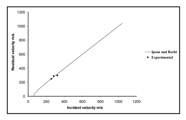
Fig. 8. Final velocity V(r) versus incident velocity V(i) for 4 layer woven composite by hemispherical projectile
