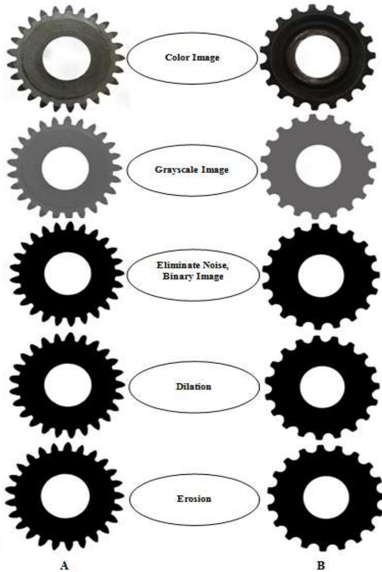
Figure (6) Samples (A, B) of Spur Gears
