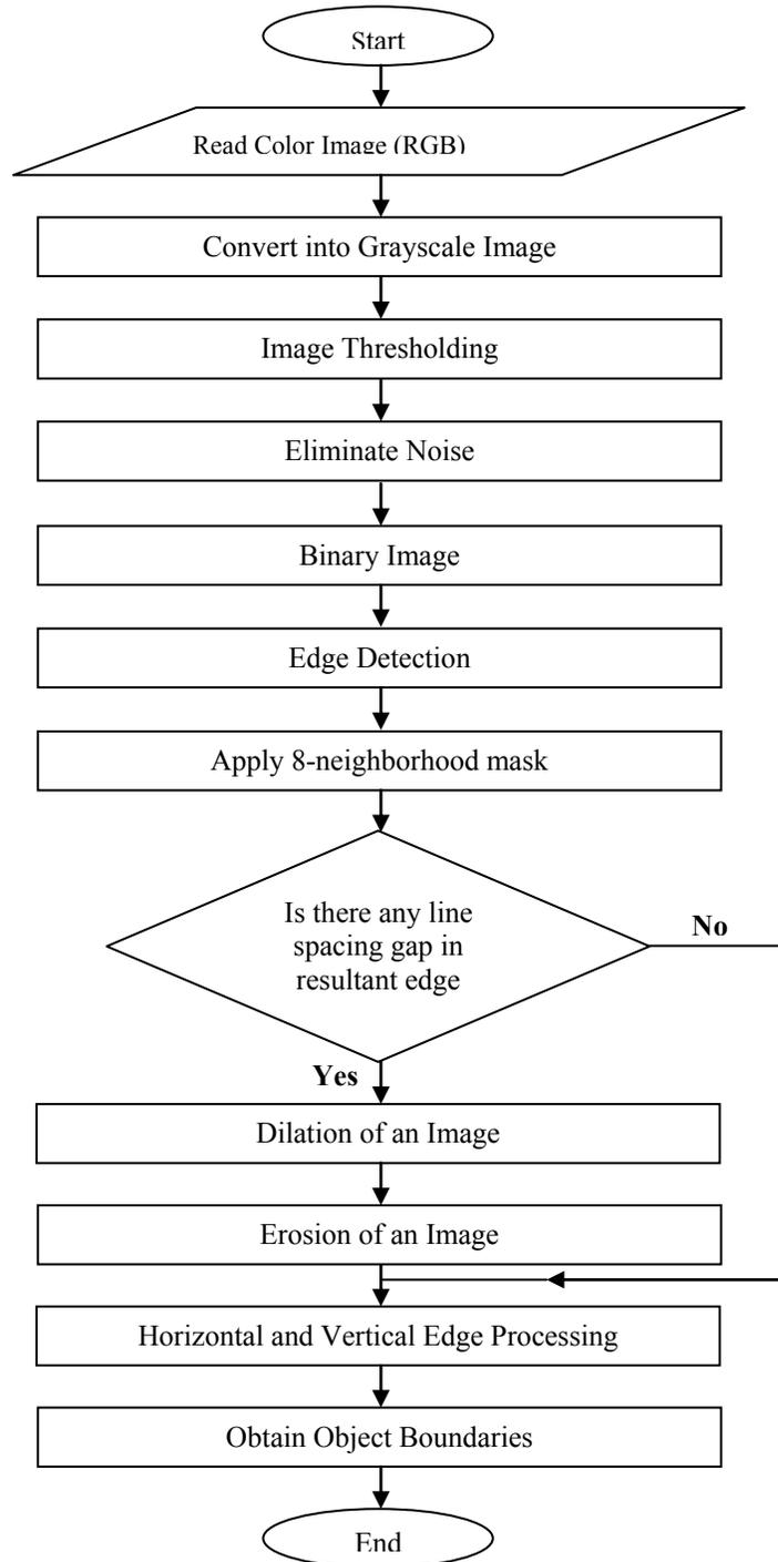
**Figure (5) The flow chart of the proposed algorithm**
