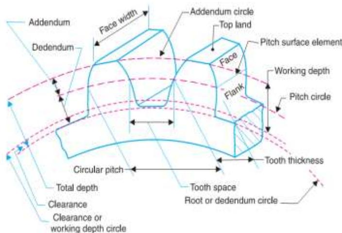
**Figure (2): Spur gear terminology [13].****Digital Image Processing (DIP)**
