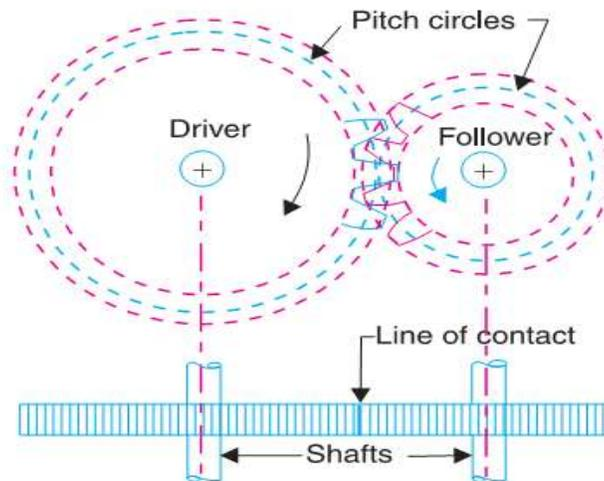
Figure (1) Spur Gear [13]
