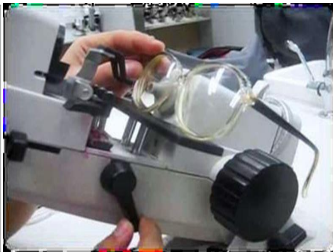
Fig. (4): Method for measuring lens power.
