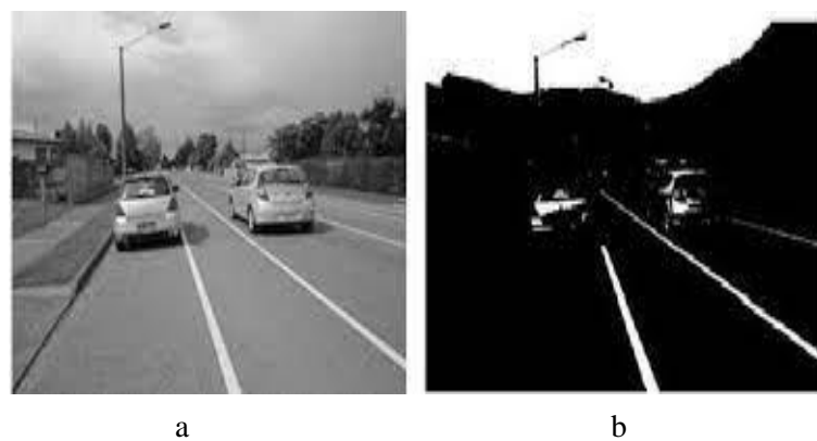
FIG. 4. PREPROCESSING IMAGES A) GRAYSCALE, B) BINARY.
