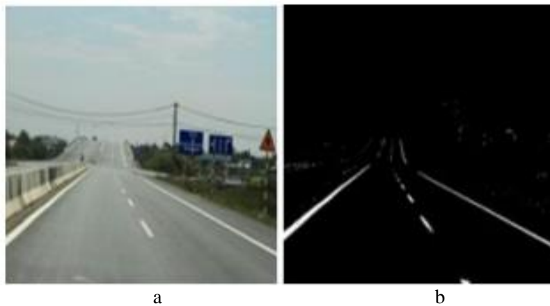
FIG. 8. DETECTED LANES BY HIS COLOR MODEL A) INPUT IMAGE, B) DETECTED LANES.
