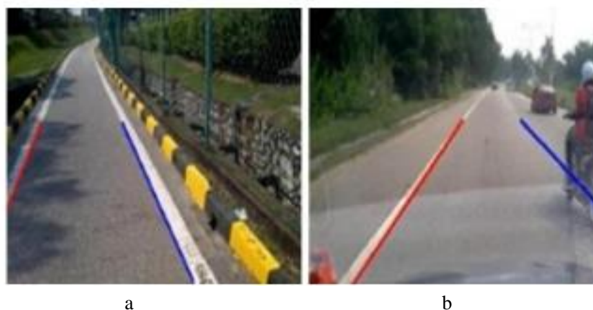
FIG. 9. RESULT OF LANE DETECTION A) SHADOWS, B) VEHICLES.
