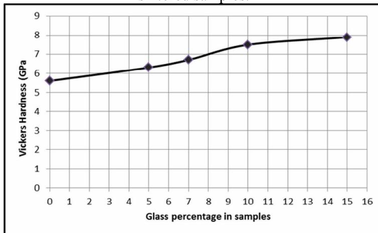
Figure(2) Effect of additive percentage of glass on Vickers hardness for the sintered samples.
