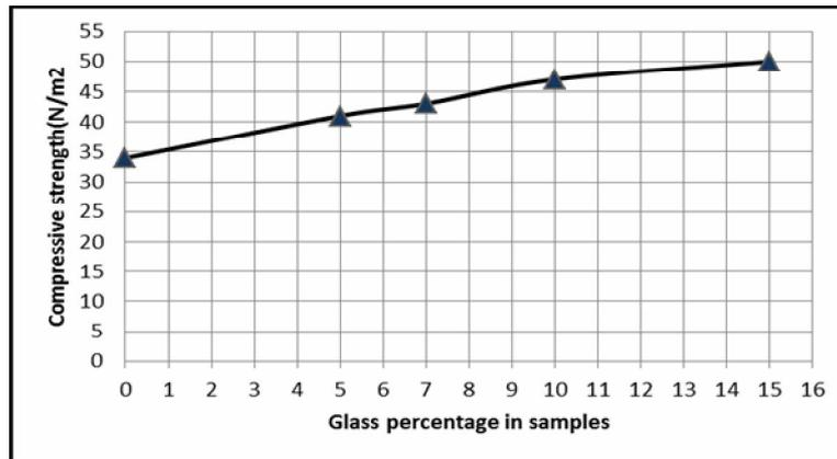
Figure(1) Effect of additive percentage of glass on compressive strength for the sintered samples.
