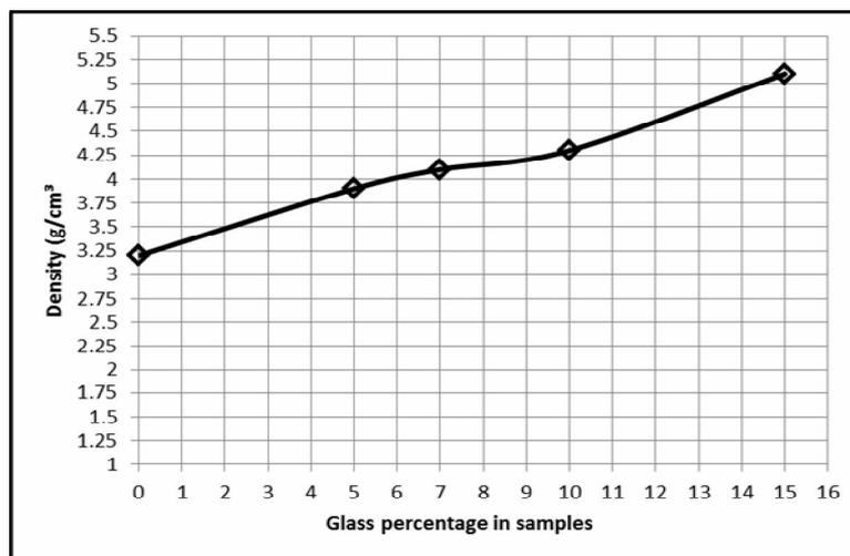
Figure(3) Effect of additive percentage of glass on bulk density for the sintered samples.
