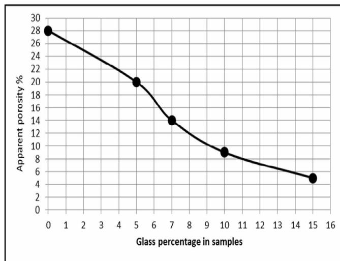
Figure(4) Effect of additive percentage of glass on apparent porosity for the sintered samples.
