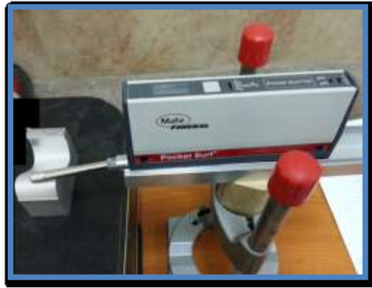
Figure (6): Measuring surface roughness by Pocket Surf tester
