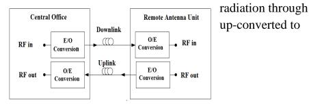
Figure 2: Radio over Fiber System Architecture. [9]
