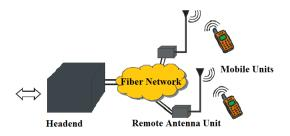
Figure 1: Radio over Fiber System Concept. [9]
