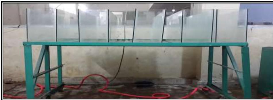
Figure (2): Containers to measure water from outlets
