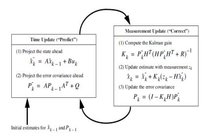
Figure 1 Complete picture of operation of Kalman filter [4]6. the proposed
