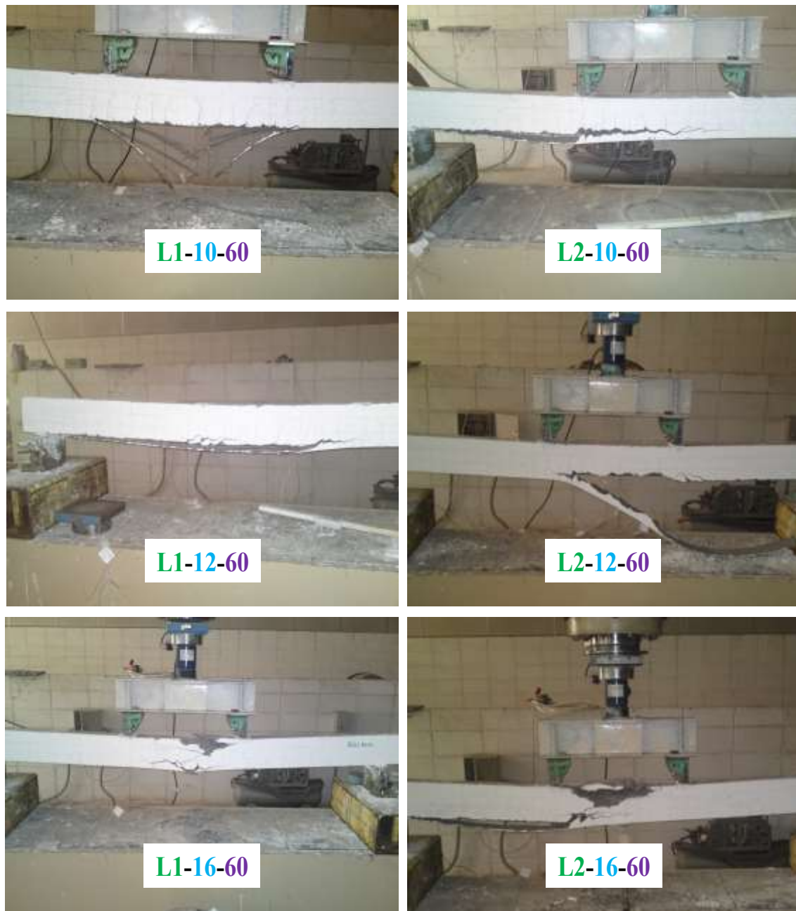
Figure. (7) Mode of failure for all beams
