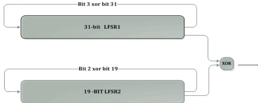
Figure (4).LFSR (Register 32bit and Register 19 bit)
