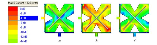
Fig. 7. Current density distribution at the surface of the first iteration microstrip bandpass filter with slots simulated at frequency of (a) 2.3 GHz, (b) 2.4 GHz, and (c) 2.5 GHz.
