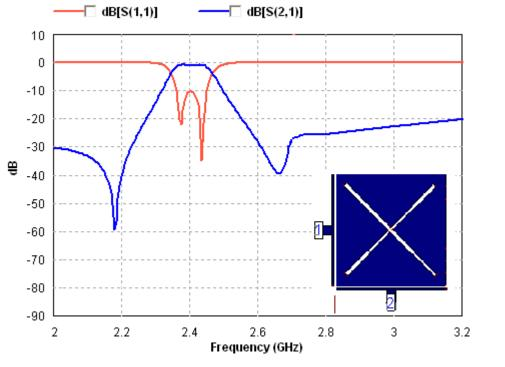
return loss and transmission responses of the dual-mode microstrip square patch resonator depicted in Fig. 2b.
