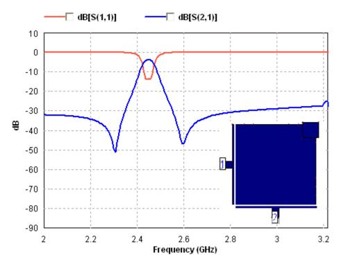
fig3.the return loss and transmission responses of the dual-mode microstrip square patch resonator depicted in Fig.2a.
