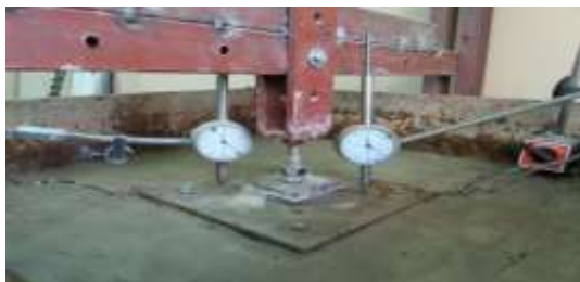
Figure 8: Loading of piled raft test
