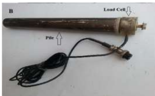
a - Load cell at pile tip- b - Load cell at pile head. Figure 3: Instrumented model piles with load cells.
