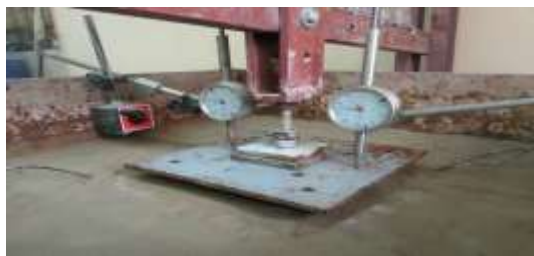
Figure 9: Loading of freestanding pile group test
