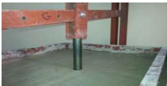
Figure 6: Installation of model piles in the clay
